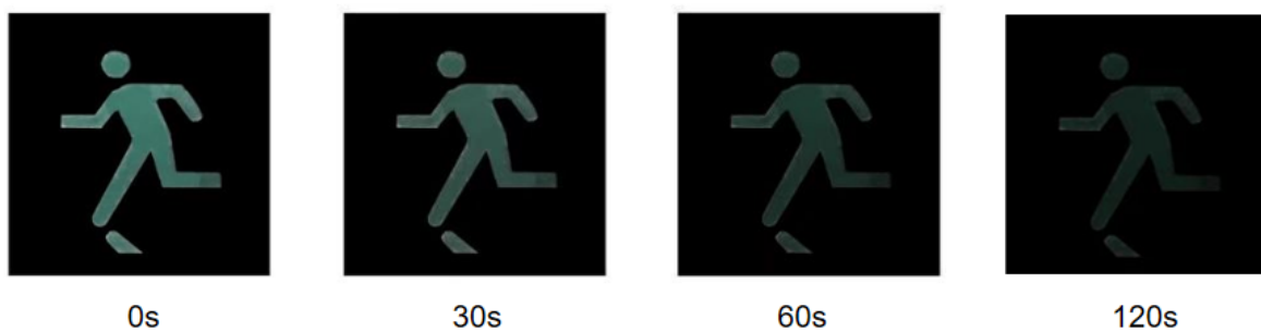
Figure S9. Time-sequence images of the "Emergency Exit" sign after UV light cessation (at 0, 30, 60, and 120 s).
