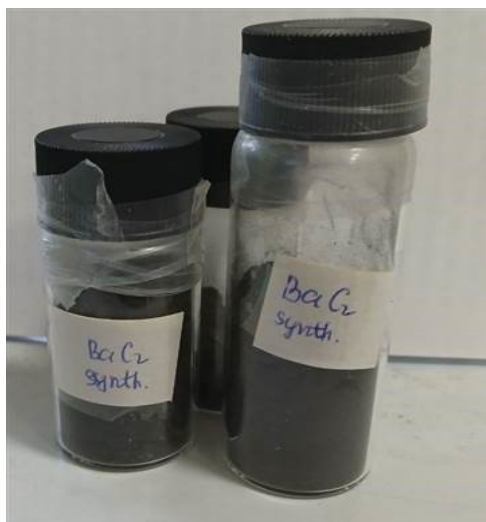
Figure S1. Barium carbide synthesized from elemental Ba and graphite at 600 °C.
