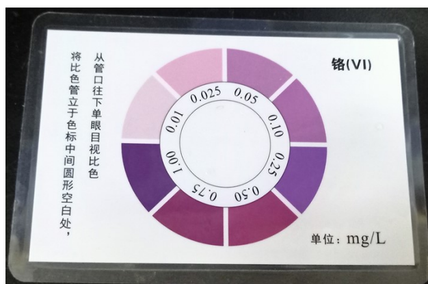
Fig. S15 Schematic diagram of Cr(VI) detection card
