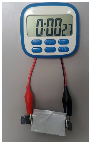
Fig. S21. Digital photographs showing the application of Zn|PAAHE|CPC ZHC in the electronic timer.
