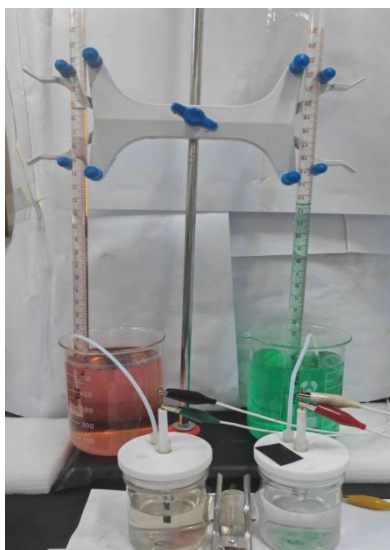
Fig. S12 Optical photographs of H 2 and O 2 collected by drainage method.
