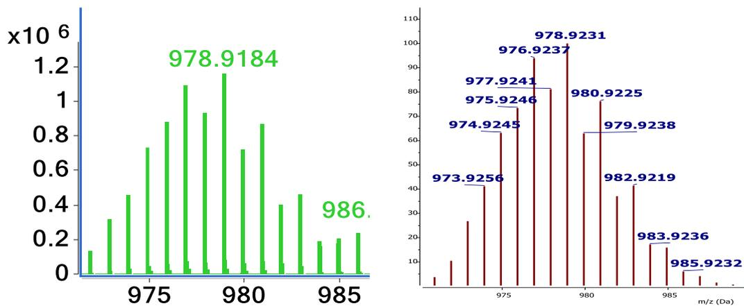
**Figure S13C.** HRMS(ESI) expanded (left) Simulated (right) spectra of **3** at  $m/z$  978.9184
