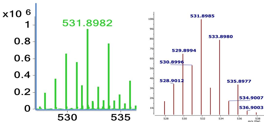
Figure S15B. HRMS(ESI) expanded (left) Simulated (right) spectra of **5** at  $m/z$  531.8982
