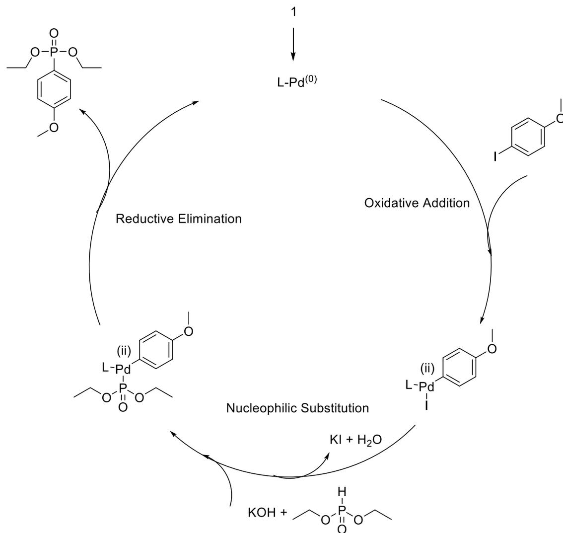
**Scheme S1:** Proposed mechanism for C-P bond formation between 4-iodoanisole and diethylphosphite catalyzed by catalyst **1**.
