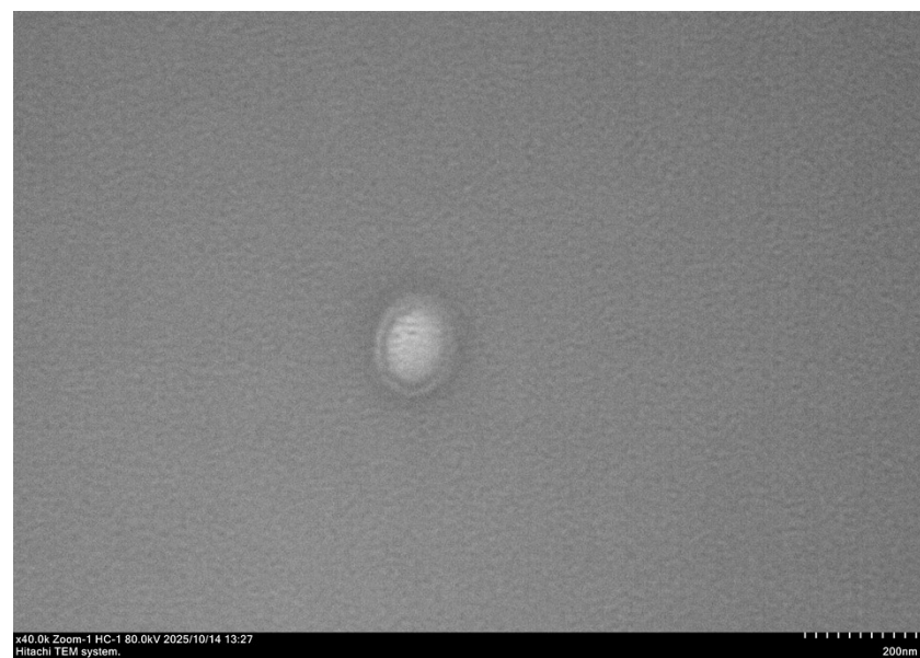
Figure S102. TEM imaging of SPC/Ch/PEG/3g-liposomes, a stock diluted 1000 times in 10 mM Tris buffer, pH = 7.4.
