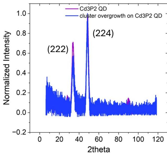
**Figure S6.** Powder X-ray diffraction of  $\text{Cd}_3\text{P}_2$  QDs on the  $\text{Co-K}\alpha$  line before and after cluster overgrowth. The characteristic (222) and (224) peaks<sup>1-3</sup> indicate the tetragonal crystal structure is preserved.
