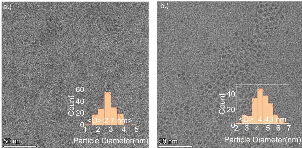
**Figure S4.** TEM images of overgrowth treatment of 1025 nm emitting QDs: (a) initial QDs with average size of 2.7 nm (b) final QDs with average size 4.4 nm
