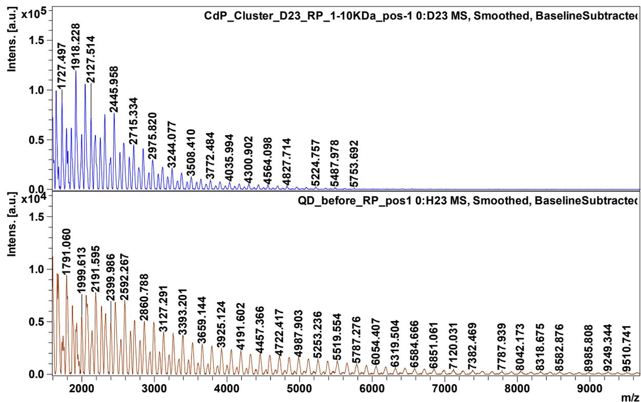
**Figure S1.** MALDI MS spectrum of cadmium phosphide MSCs and QDs emitting at 1010 nm taken in the positive reflectron mode using matrix DCTB in the 1:1 sample: matrix ratio of (a) MSCs and (b) QDs.
