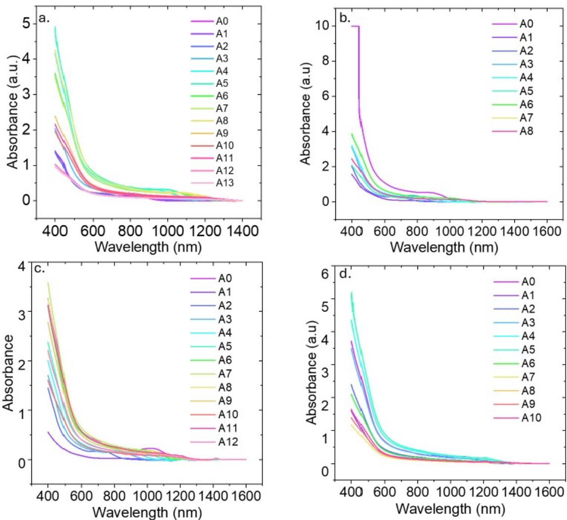
**Figure S2.** Absorption spectra of cluster overgrowth trials on (a) 965 nm emitting QDs, (b) 1010 nm emitting QDs, (c) 1102 nm emitting QDs, and (d) 1145 nm emitting QDs.
