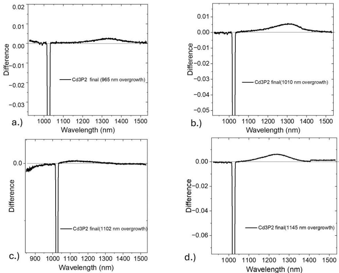
**Figure S3.** PLQY of the final product of the cluster overgrowths on (a) 965 nm, (b) 1010 nm, (c) 1102 nm, and (d) 1145 nm emitting QDs.
