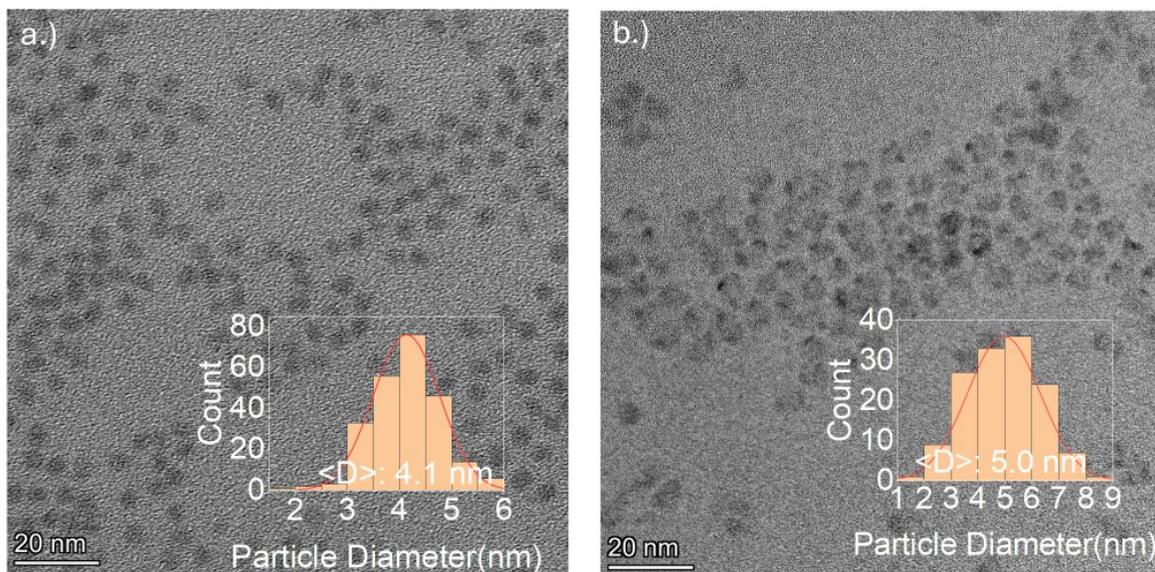
**Figure S5.** TEM images of overgrowth treatment of 1145 nm emitting QDs: (a) initial QDs with average size of 4.1 nm (b) final QDs with average size of 5.0 nm.
