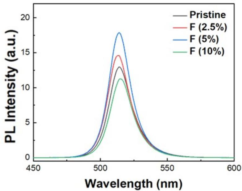
**Figure S4.** The unnormalized PL spectra under different NaPF<sub>6</sub> doping
