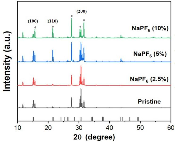
**Figure S3.** The X-ray diffraction (XRD) patterns with different NaPF<sub>6</sub> doping
