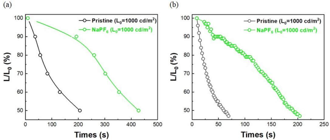
**Figure S10.** The device lifetime ( $T_{50}$ , initial luminance of  $1000 \text{ cd/m}^2$ ) of pristine and  $\text{NaPF}_6$ -treated device (a) package, (b) unpackaged
