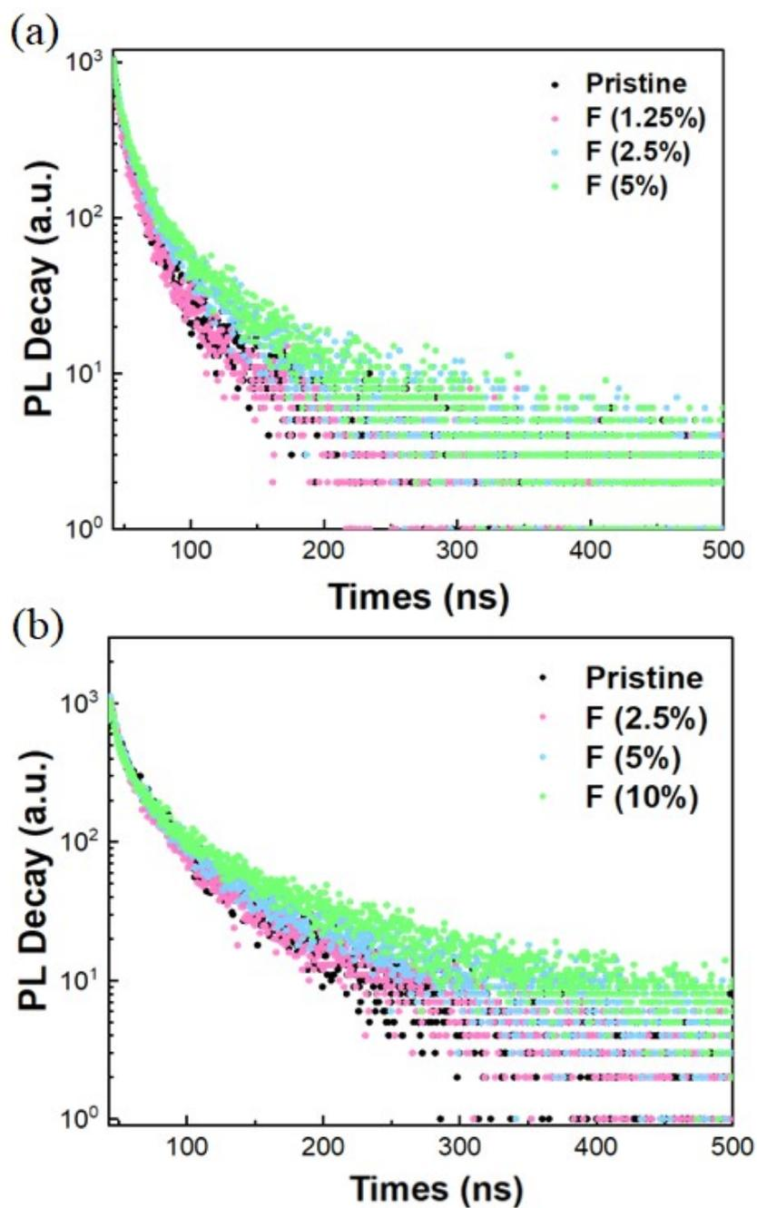
**Figure S5.** (a) The PL Decay of sky blue (490 nm) perovskite films, (b) The PL Decay of pure blue (474 nm) perovskite films
