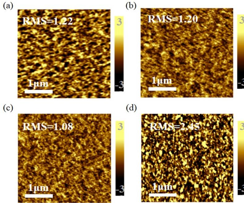
**Figure S1.** The films' atomic force microscopy (AFM) images by different  $\text{NaPF}_6$  doping concentrations (2.5%, 5%, 10%)
