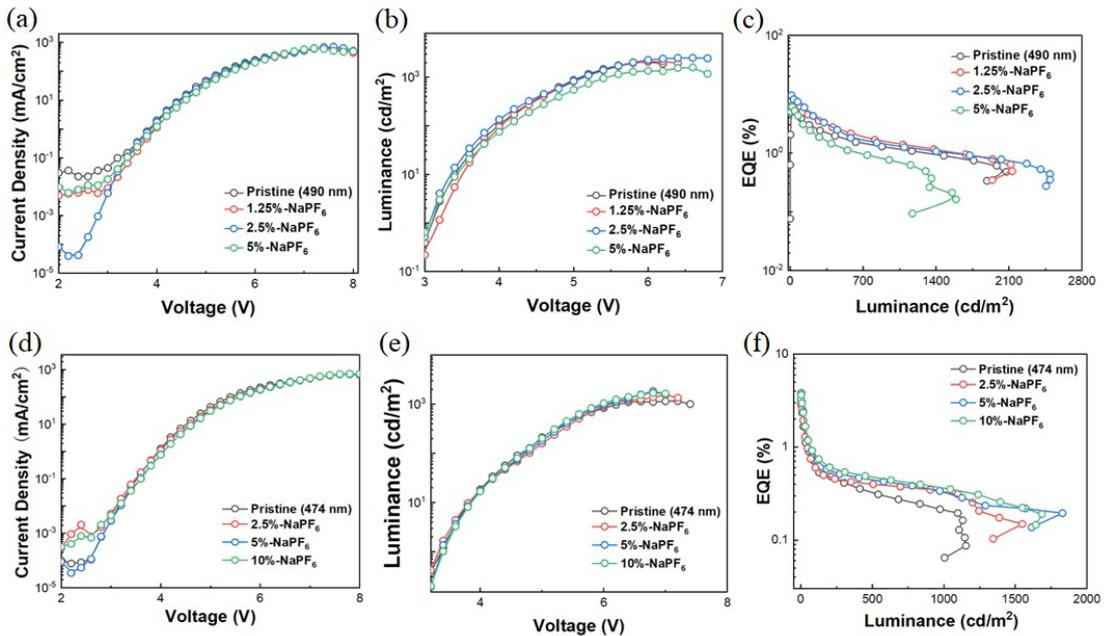
**Figure S11.** (a) Current density-voltage (J-V) curves, (b) Luminance- voltage (L-V) curves, (c) EQE-luminance (EQE-L) curves of sky blue PeLEDs at different  $\text{NaPF}_6$  doping. (d) Current density-voltage (J-V) curves, (e) Luminance- voltage (L-V) curves, (f) EQE-luminance (EQE-L) curves of pure blue PeLEDs at different  $\text{NaPF}_6$  doping.
