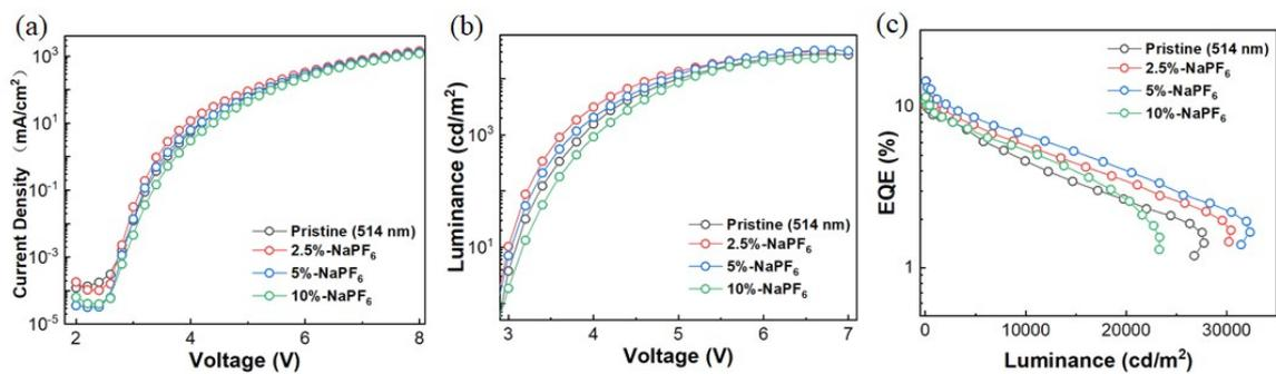
**Figure S9.** (a) Current density-voltage (J-V) curves, (b) Luminance- voltage (L-V) curves, (c) EQE-luminance (EQE-L) curves of green PeLEDs at different NaPF<sub>6</sub> doping
