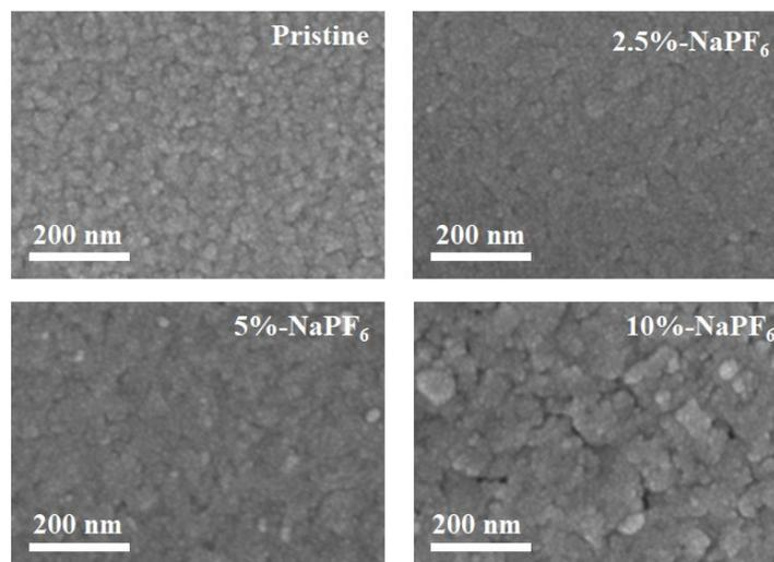
**Figure S2.** The SEM images of perovskite films at different  $\text{NaPF}_6$  doping concentrations (pristine, 2.5%, 5%, 10%)
