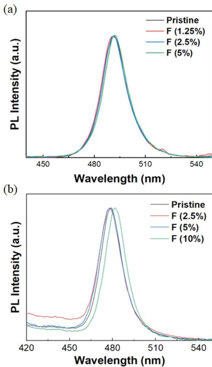
**Figure S6.** (a) The sky blue PL spectra with different NaPF<sub>6</sub> doping, (b) The pure blue PL spectra with different NaPF<sub>6</sub> doping
