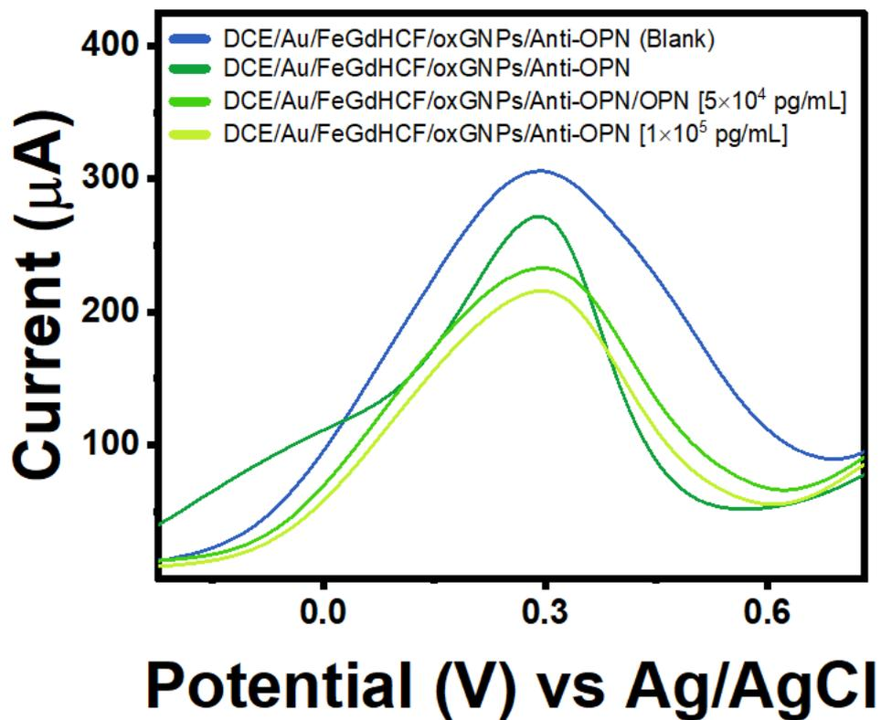
**Fig. SI 3:** DPV responses recorded on a disposable printed carbon electrode (DCE) showing Blank (blue), DCE/Au/FeGdHCF/oxGNPs/Anti-OPN (dark green), DCE/Au/FeGdHCF/oxGNPs/Anti-OPN/OPN for two concentrations:  $5 \times 10^4$  pg/mL (light green) and  $1 \times 10^5$  pg/mL (lime).
