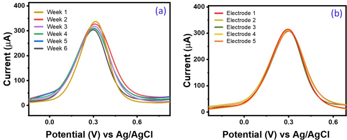
**Fig. SI 2:** DPV curves showing (a) durability and stability of the immunosensor probe to detect OPN [Conc.  $1 \times 10^4$  pg/mL] over six weeks (b) reproducibility of the sensing probe by studying current responses using five separate electrodes under same operational parameters.
