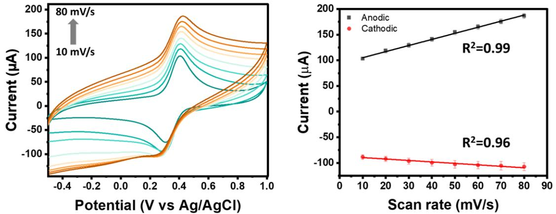
**Fig. SI 1:** CV responses and corresponding linear plot showing the scan rate study (10-80 mV/s) of GCE/Au/FeGdHCF/oxGNPs/Anti-OPN in 5mM PBS [ $I_{pa}=93.18 (\pm 1.06) + 1.18 (\pm 0.02) \text{Scan rate (mV/s)}$ ] and  $I_{pc} = -86.59 (\pm 0.01) + \{-0.28 (\pm 0.02)\} \text{Scan rate (mV/s)}$ ]
