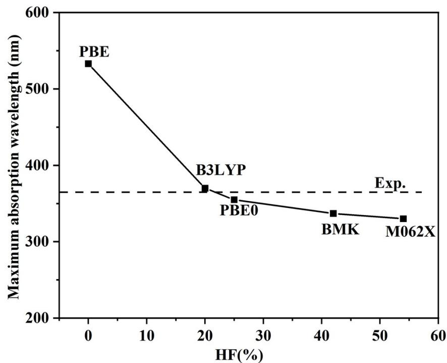
**Figure S1.** (a) The lowest unoccupied orbital (LUMO) energy and (b) maximum absorption wavelength of NDIN with different functionals. The dashed lines indicate the experimental values.
