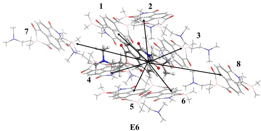
**Figure S2.** The predicted crystal structures and the main electron hopping pathways of the investigated molecules.
