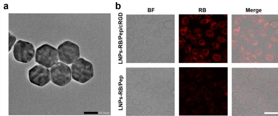
**Figure S13.** (a) TEM Image of LNP-RB/Pep/cRGD. Scale bar: 50 nm. (b) Confocal microscopic images of HCCLM3 cells incubated with LNP-RB/Pep/cRGD (200  $\mu\text{g}/\text{mL}$ ) and LNP-RB/Pep (200  $\mu\text{g}/\text{mL}$ ) for 4h respectively. Scale bar: 75  $\mu\text{m}$ .
