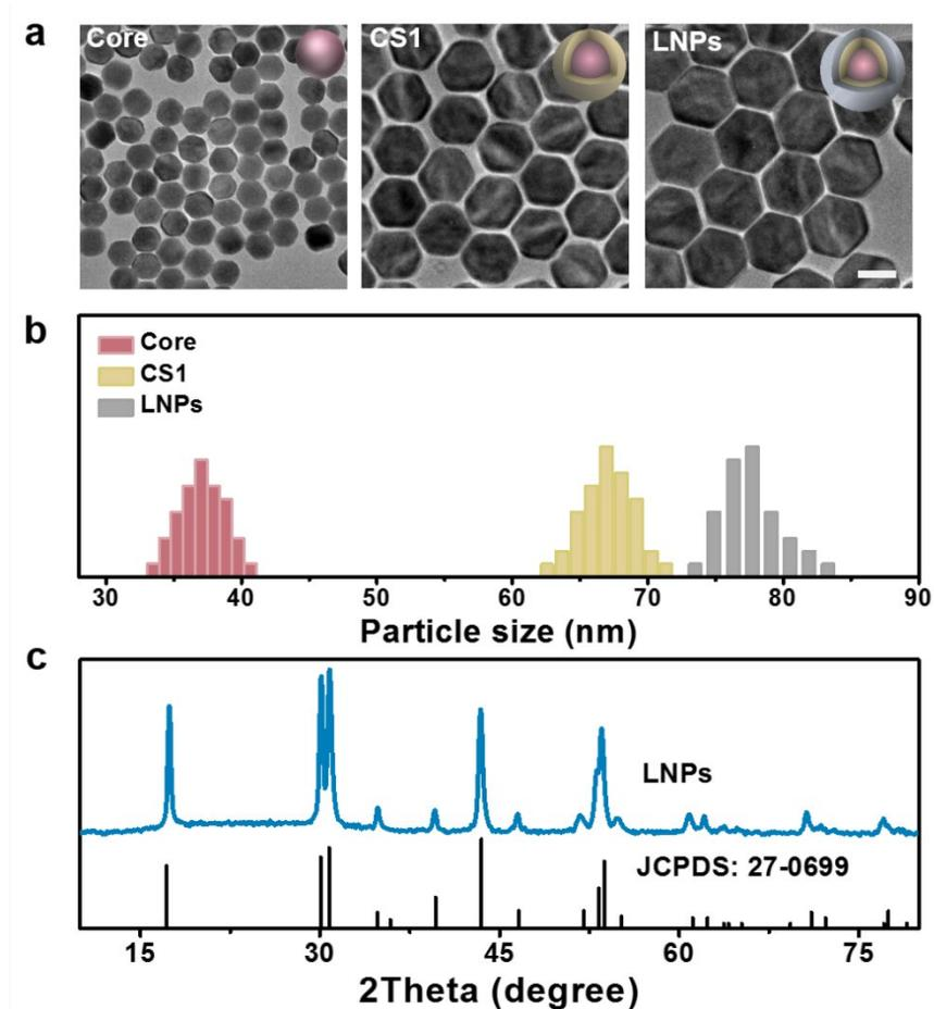
**Figure S1.** (a) TEM images and (b) size distribution of LNP NaGdF<sub>4</sub>:Yb,Er,Ce (core), layered structure NaGdF<sub>4</sub>:Yb,Er,Ce@NaYbF<sub>4</sub>:Nd (CS1), and NaGdF<sub>4</sub>:Yb,Er,Ce@NaYbF<sub>4</sub>:Nd@NaGdF<sub>4</sub> (LNPs), Scale bars are 50 nm. (c) XRD patterns of LNPs and  $\beta$ -NaGdF<sub>4</sub> (JCPDS: 27-0699).
