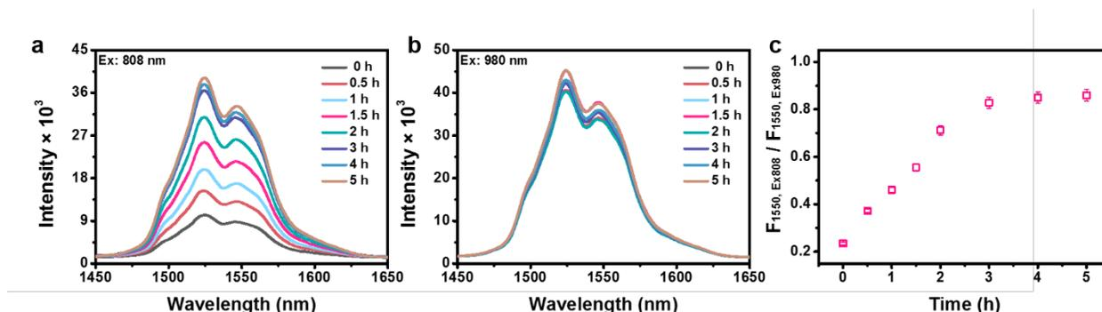
**Figure S9.** Time dependent NIR-IIb luminance spectra of LNPs-RB/Pep (2 mg/mL, 500 μL) with caspase-3 (8 U/mL) incubation different times (0-5 h) at 37 °C under (a) 808 nm, (b) 980 nm excitation and (c) F<sub>1550, Ex808</sub> / F<sub>1550, Ex980</sub> ratio change.
