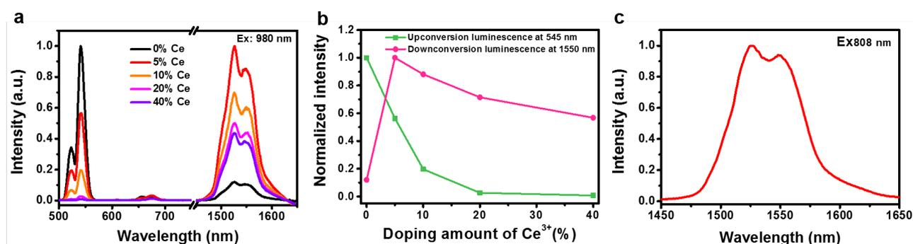
**Figure S2.** (a) Upconversion and downconversion luminescence spectra of NaGdF<sub>4</sub>:Yb,Er,Ce (Ce% = 5, 10, 20, 40) under 980 nm excitation and (b) their corresponding normalized luminescence intensity. (c) Downconversion luminescence spectrum of LNPs under 808 nm excitation.
