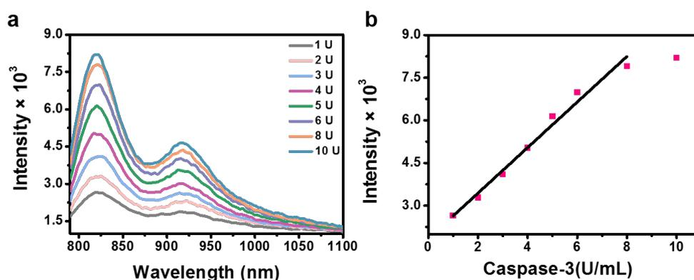
**Figure S11.** Fluorescence emission spectra of supernatant for LNPs-RB/Pep (2 mg/mL, 500  $\mu$ L) incubating with different concentrations caspase-3 (1-10 U/mL) at 37  $^{\circ}$ C for 3h and (b) the linear relationship between emission peak intensity at 820 nm corresponding to caspase-3 concentration.
