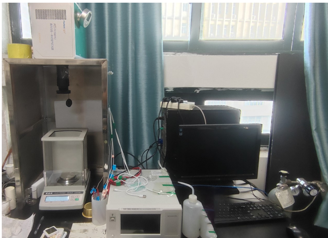
Figure. S7. Photographs of xenon lamp desorption equipment.
