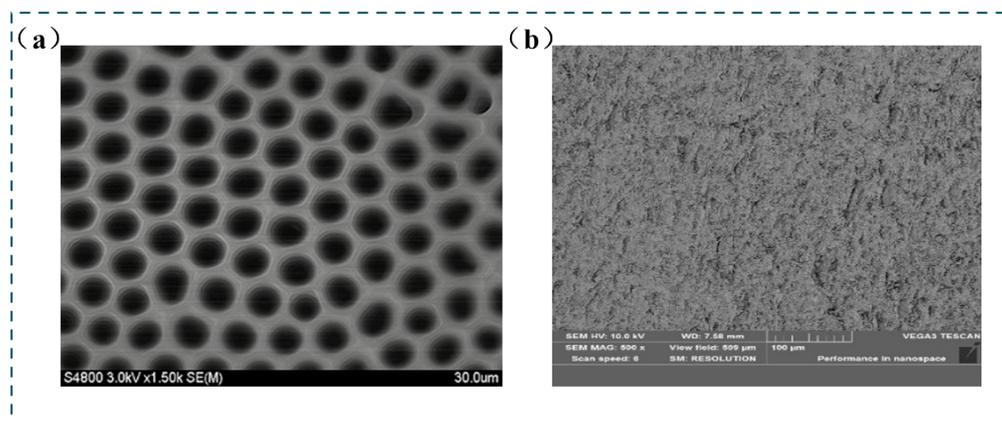
Fig. S1. (a) SEM image of AAO template (b) SEM image of PR/PDMS
