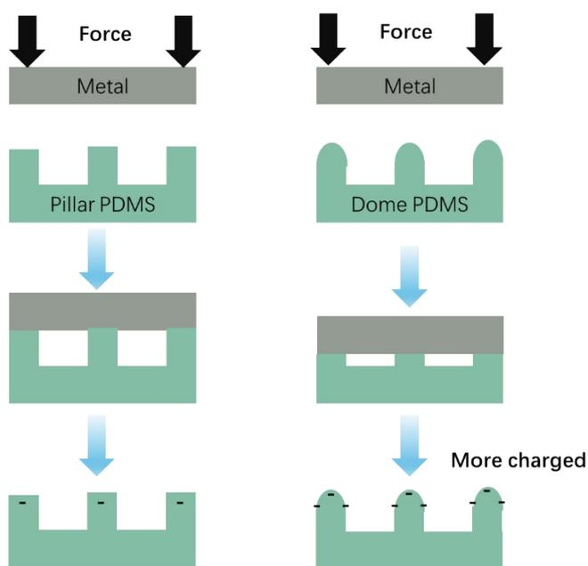
Figure S4: Effect of protruding surface shapes on the performance of the friction layer in contact-separation mode
