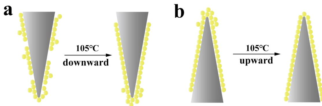
**Fig. S1** Schematic diagram of aggregation of Au nanoparticles in the apex after tip is annealed in a downward direction (a), departure of excess Au nanoparticles from the apex after tip is annealed in a upward direction (b).
