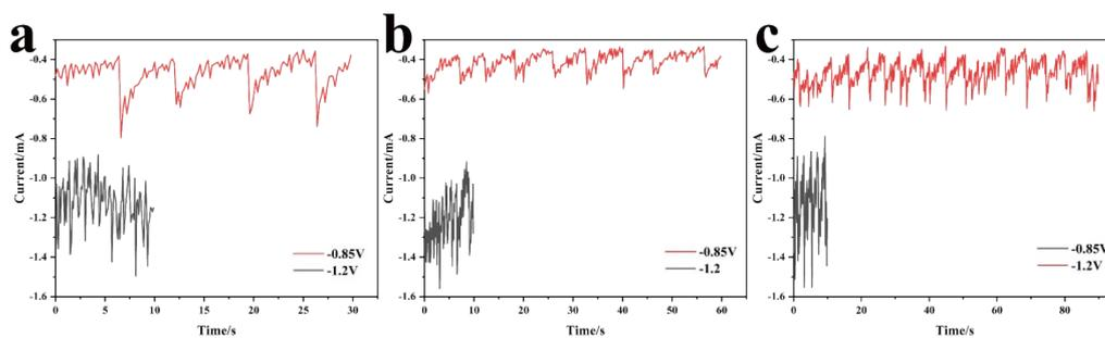
**Fig. S5** Current-time curves of electrodeposition using potentiostatic method on the surface of annealed Au nanoparticles film modified tip. The initial deposition is performed at -1.2 V for 10 s, and followed by deposition at -0.85 V for 30 s (a), 60 s (b) and 90 s (c), respectively.
