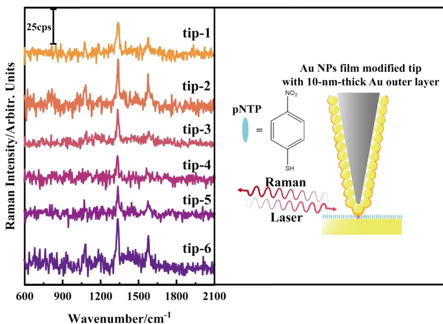
**Fig.S6** TERS spectra of pNTP obtained by different Au nanoparticles film modified tips with 10-nm thick Au outer layer. The spectra are recorded using a 638 nm laser with a power of 0.13 mW and an acquisition time of 1 s.
