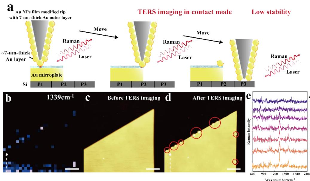
**Fig. S8** Schematic diagram of Au nanoparticles film modified tip with 7-nm thick Au outer layer for TERS imaging in contact mode (a). TERS image of band intensity at 1339 cm<sup>-1</sup> of pNTP (b). In-situ AFM images of Au MP before (c) and after (d) TERS imaging. The scale bar is 1 μm. TERS spectra are collected at the positions marked by the dotted line in the images. The spectra are recorded using a 638 nm laser with a power of 0.13 mW and an acquisition time of 1 s (e).
