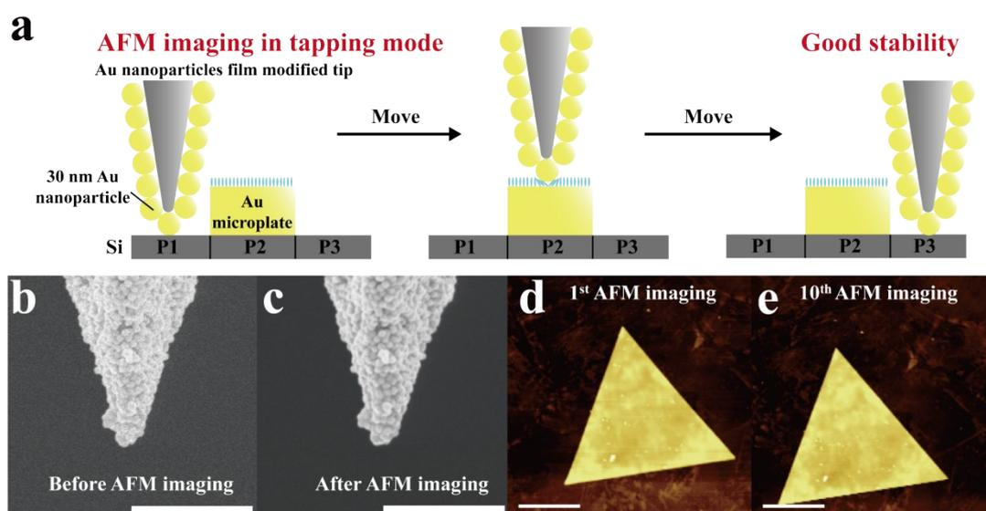
**Fig. S7** Schematic diagram of annealed Au nanoparticles film modified tip for AFM imaging in tapping mode (a). SEM images of annealed Au nanoparticles film modified tip are recorded before (a) and after (b) AFM imaging. The scale bar is 500 nm. AFM images of the Au MP after 1<sup>st</sup> (c) and 10<sup>th</sup> (d) scanning by the annealed Au nanoparticles film modified tip. The scale bar is 2  $\mu\text{m}$ .
