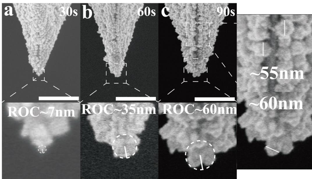
**Fig. S4** SEM images of Au nanoparticles film modified tip with Au outer layer prepared at the initially deposition potential of -1.2 V for 10 s, followed by positive movement of potential to -0.85 V for 30 s (a), 60 s (b) and 90 s (c). The scale bar is 500 nm.
