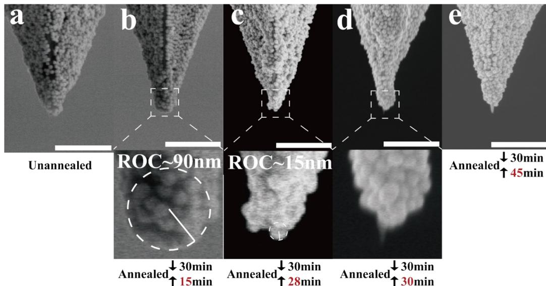
**Fig.S2** SEM images of Au nanoparticles film modified tip without annealing (a), with annealing downward for 30 min and then upward for 15 min (b), 28 min (c), 30 min (d) and 45 min (e). The scale bar is 500 nm.
