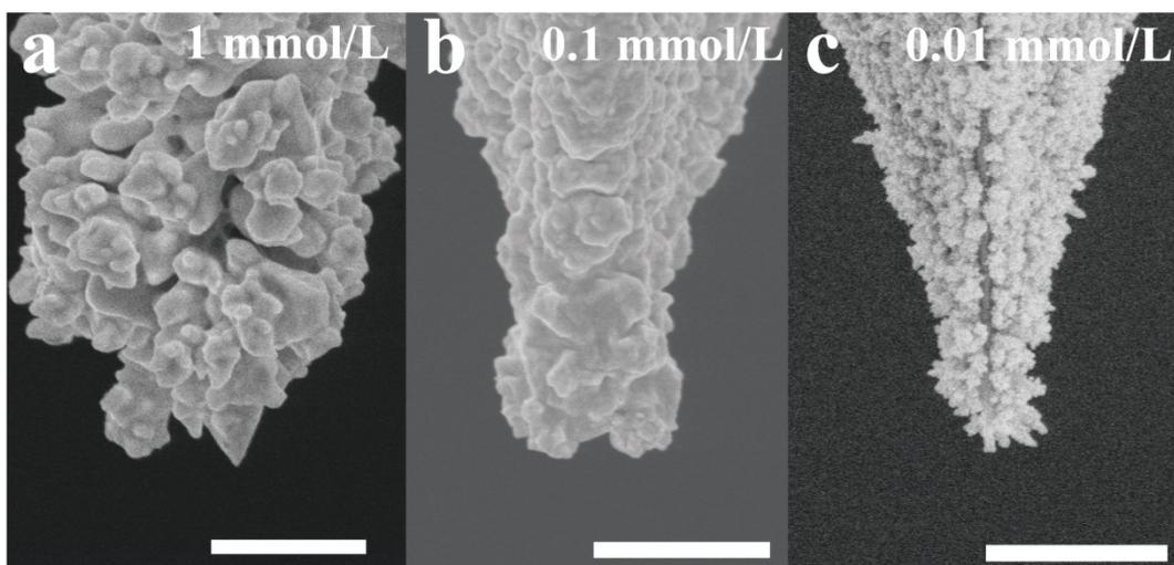
**Fig. S3** SEM images of Au nanoparticles film modified tip with Au outer layer prepared by electrodeposition with different concentration of HAuCl<sub>4</sub>: 1 mmol/L (a), 0.1 mmol/L (b) and 0.01 mmol/L (c). Potential: 0 to -1.4 V, scan rate: 50 mV/s. The scale bar is 500 nm.
