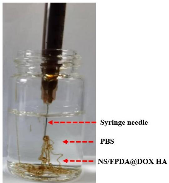
Figure S3. The injectability of NS/FPDA@DOX HA in PBS solution.
