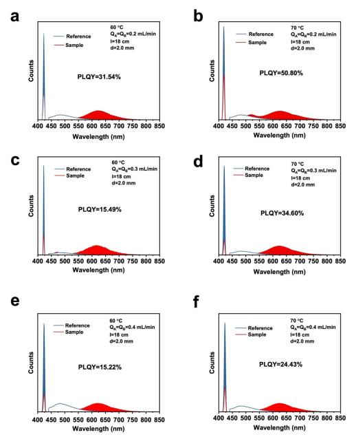
PL spectra of CdS:Ag<sup>+</sup> doped-QDs synthesized using batch flask method, MPB and tube microreactor without MPB.
