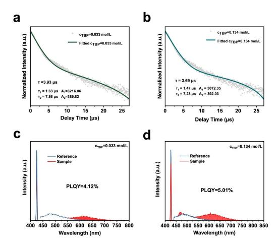
Excitation light on reference toluene ( $\lambda_{ex}$  = 365 nm) and PL spectrum of CdS:Ag<sup>+</sup> QDs synthesized at different temperature and flow velocity.
