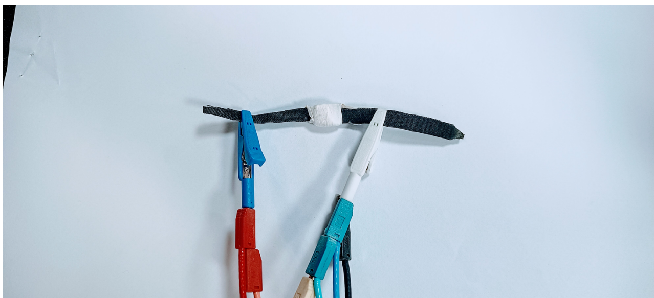
Fig. S 2 The assembled flexible asymmetric quasi-solid state supercapacitor device with the crocodile clip.
