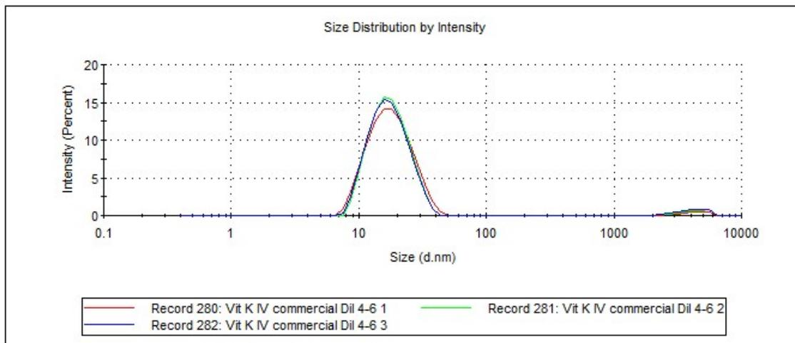
**Supplementary Figure 5.** Vitamin K1 emulsion size (Z-average) and size distribution (polydispersity index - PDI) measured by dynamic light scattering (DLS) at 22 °C with a 173 backscatter angle, using a Malvern Zetasizer Nano ZS (Malvern Instruments, Westborough, MA).
