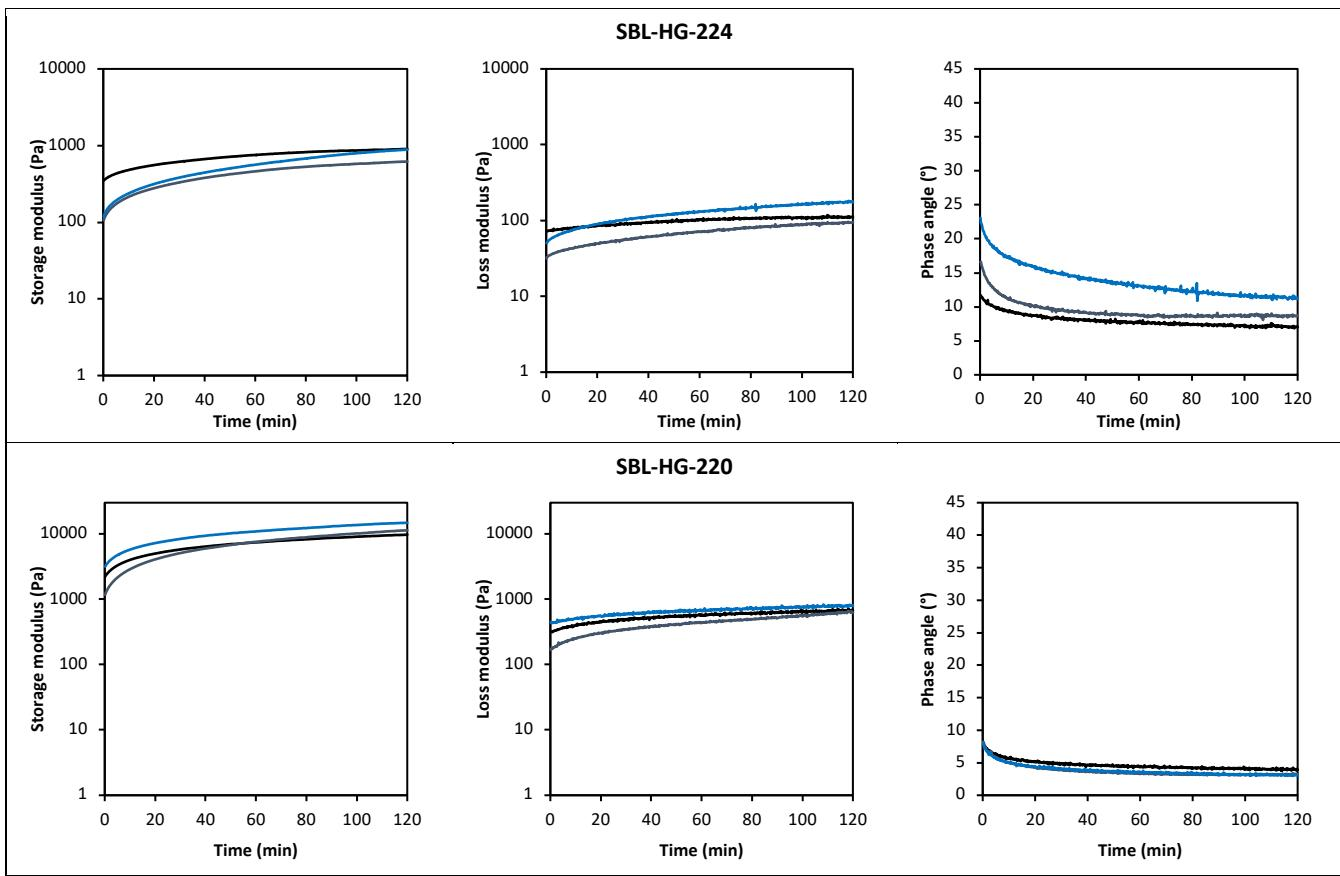
**Figure S5.** Dynamic rheology of **SBL-HG-224** and **SBL-HG-220** with storage modulus (left), loss modulus (middle) and phase angle (right) plotted as a function of time. The measurement was performed at 37°C, with a strain of 0.5% and oscillation frequency of 0.15 Hz. Colour shades represent replicate measurements.
