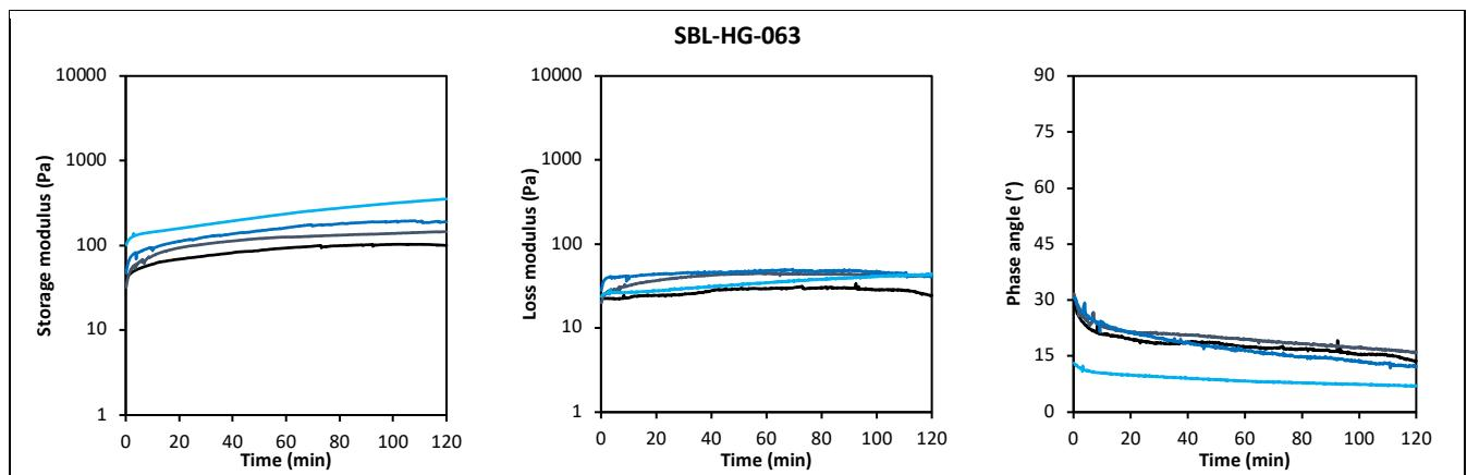
**Figure S2.** Dynamic rheology of **SBL-HG-063** with storage modulus (left), loss modulus (middle) and phase angle (right) plotted as a function of time. The measurement was performed at 37°C, with a strain of 0.5% and oscillation frequency of 0.15 Hz. Colour shades represent replicate measurements.
