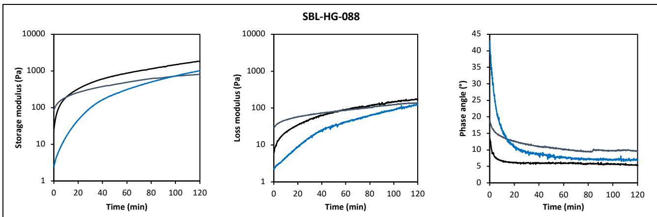
**Figure S7.** Dynamic rheology of **SBL-HG-088** with storage modulus (left), loss modulus (middle) and phase angle (right) plotted as a function of time. The measurement was performed at 37°C, with a strain of 0.5% and oscillation frequency of 0.15 Hz. Colour shades represent replicate measurements.
