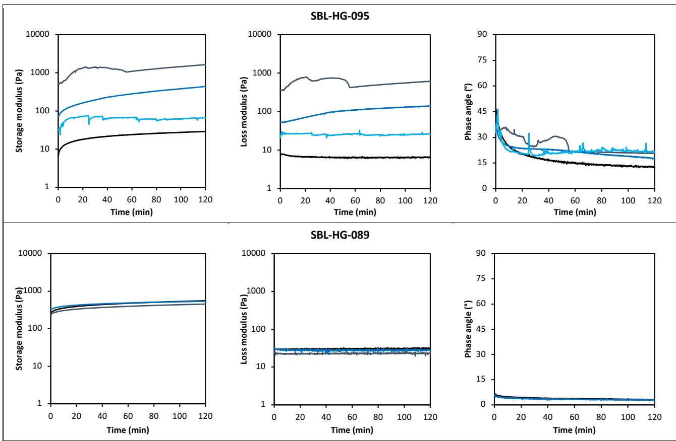
**Figure S4.** Dynamic rheology of SBL-HG-095 and SBL-HG-089 with storage modulus (left), loss modulus (middle) and phase angle (right) plotted as a function of time. The measurement was performed at 37°C, with a strain of 0.5% and oscillation frequency of 0.15 Hz. Colour shades represent replicate measurements.
