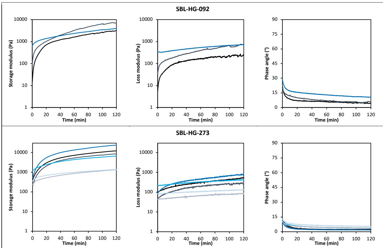
**Figure S3.** Dynamic rheology of SBL-HG-092 and SBL-HG-273 with storage modulus (left), loss modulus (middle) and phase angle (right) plotted as a function of time. The measurement was performed at 37°C, with a strain of 0.5% and oscillation frequency of 0.15 Hz. Colour shades represent replicate measurements.
