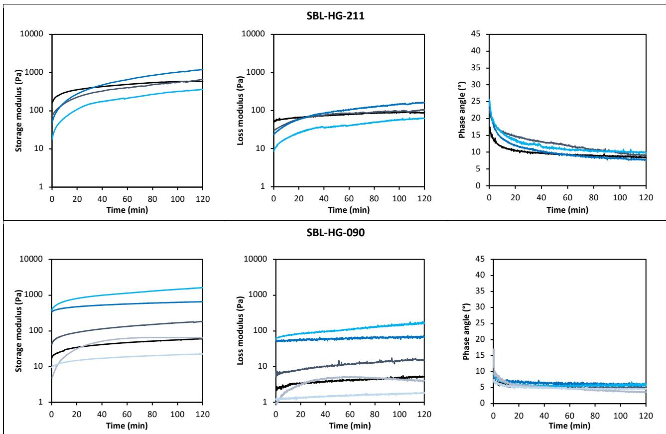
**Figure S6.** Dynamic rheology of **SBL-HG-211** and **SBL-HG-090** with storage modulus (left), loss modulus (middle) and phase angle (right) plotted as a function of time. The measurement was performed at 37°C, with a strain of 0.5% and oscillation frequency of 0.15 Hz. Colour shades represent replicate measurements.
