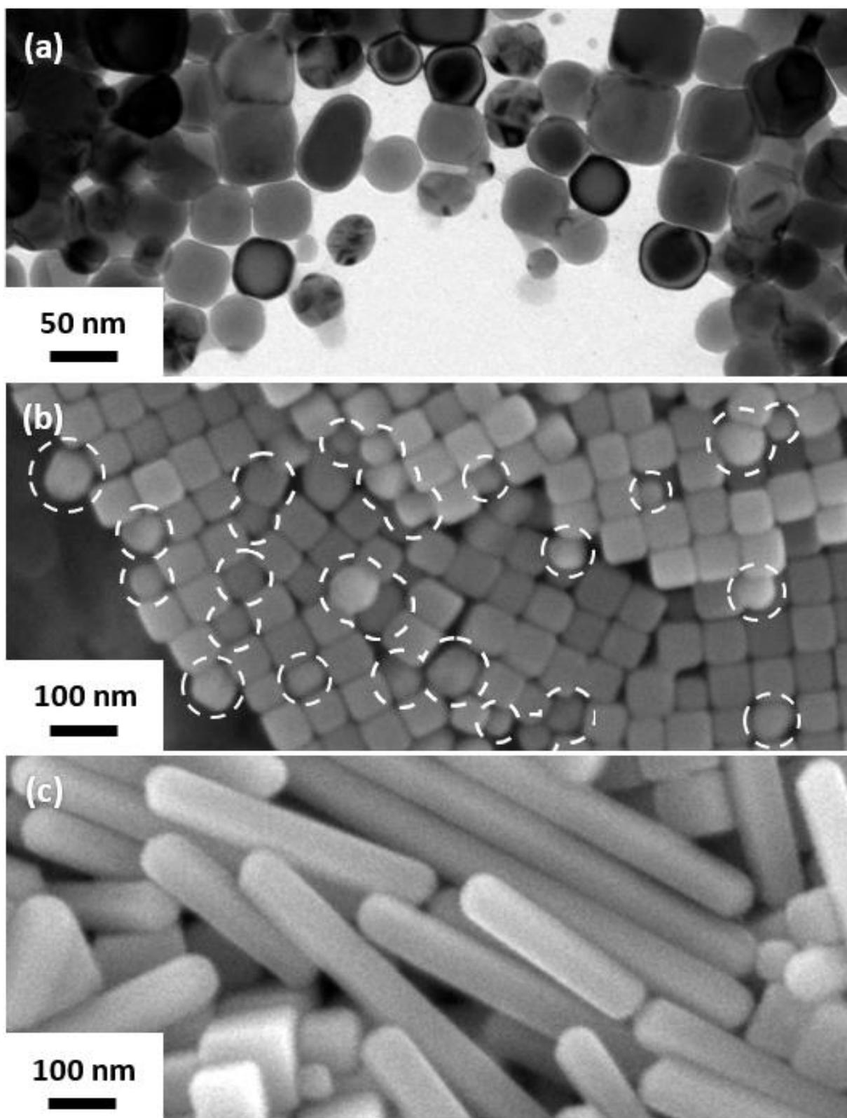
**Figure S4:** EM images of multiple twinned (MT) nanoparticles alongside single (SC) crystalline nanocubes: (a) TEM image showing a uniform contrast for SC nanocubes and a blotchy contrast for MT nanoparticles, (b) SEM image of medium-sized nanocubes and MT nanoparticles (in white dashed circles) and (c) SEM image of nanorods at high magnification.
