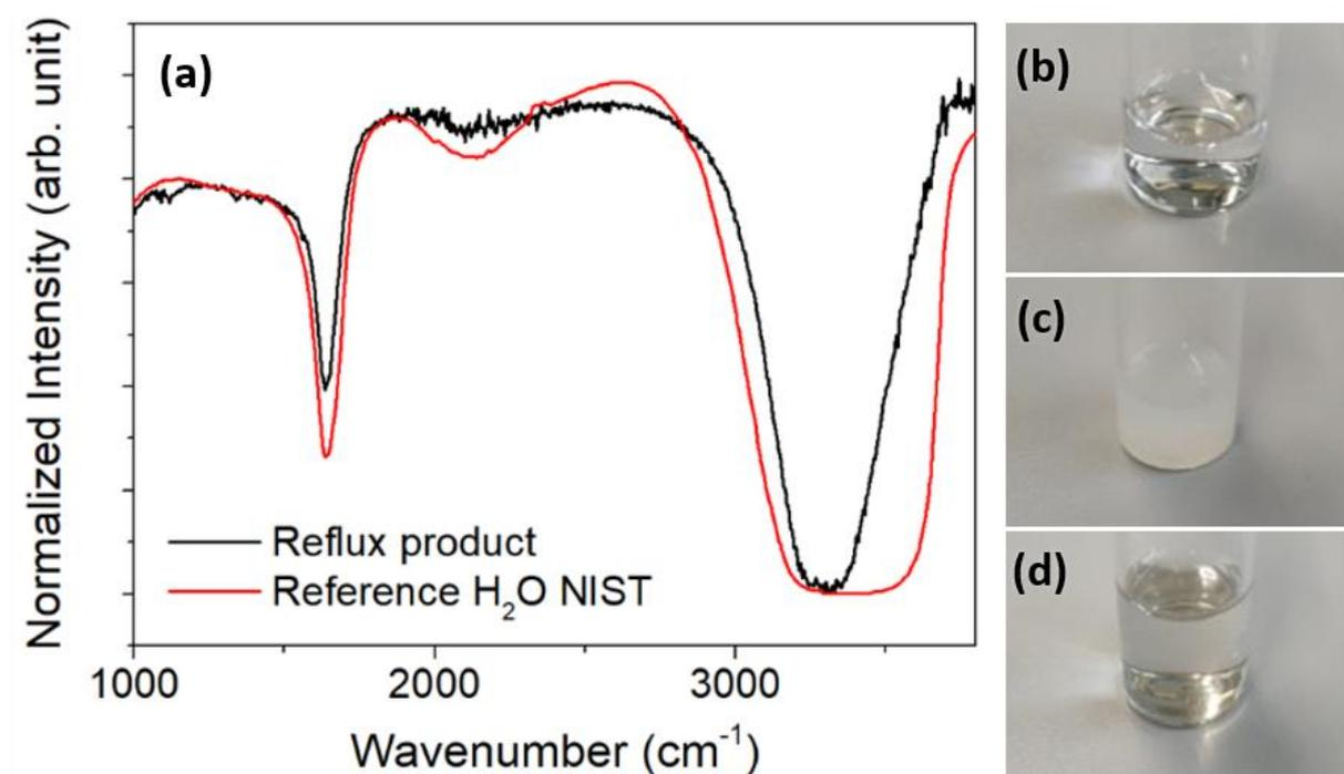
**Figure S2:** (a) IR spectrum of the reflux product and the reference spectrum of water from the NIST database as well as photographs of the chloride detection reaction:  $\text{AgNO}_3$  solution (b) before and (c) after the addition of the reflux product and (d) after a 25 %  $\text{NH}_3$  solution was added to the solution shown in image (c).
