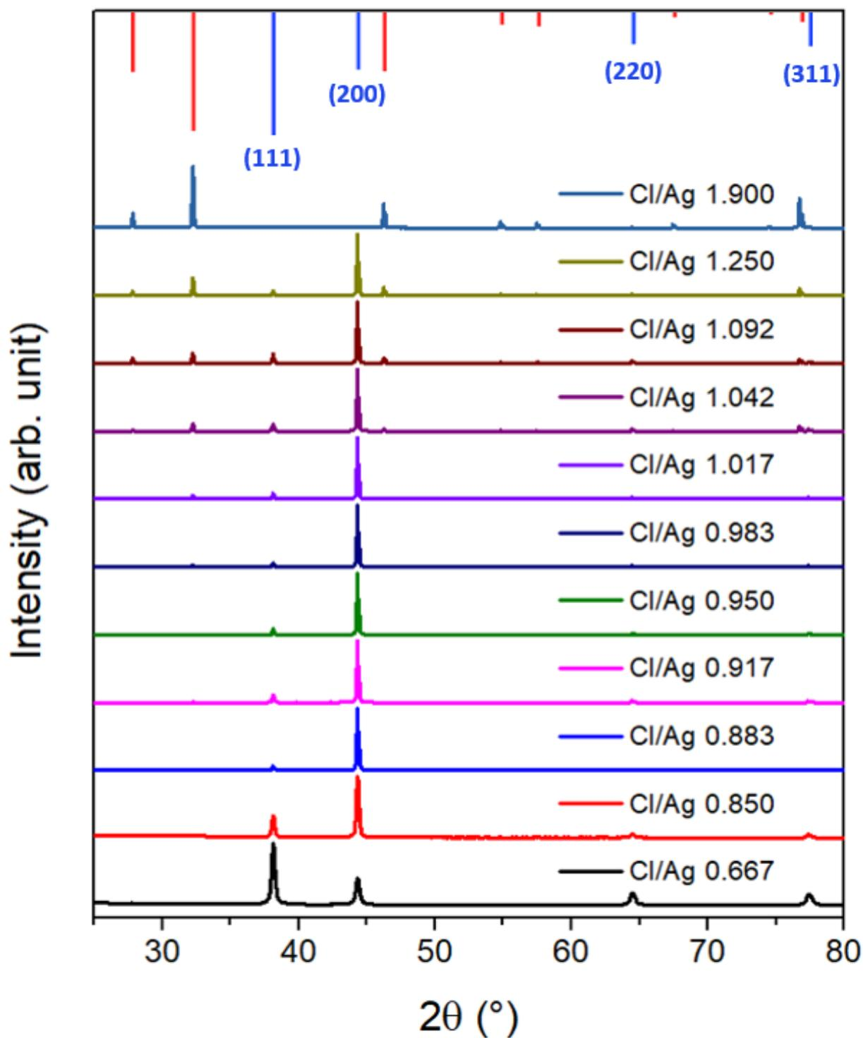
**Figure S3:** X-ray diffractograms of several samples from silver nanocube syntheses with different Cl:Ag ratios. The diffraction pattern for AgCl (COD: 9011666) is displayed in red on the top of the image, the pattern for Ag (COD: 9008459) is displayed in blue.
