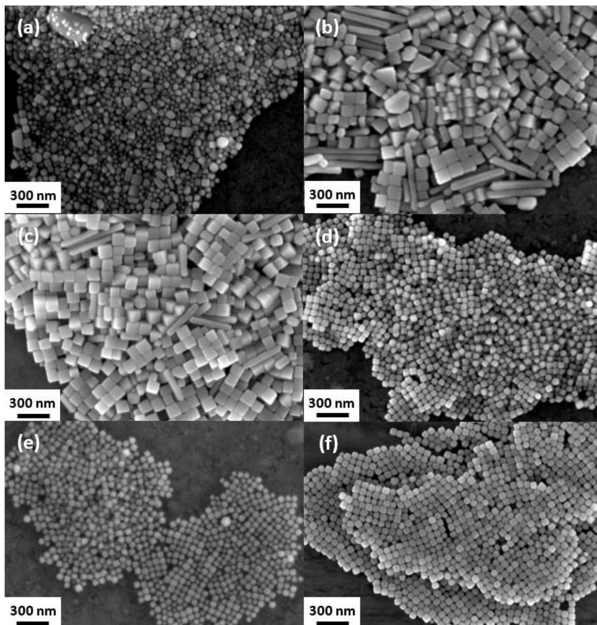
**Figure S6:** SEM images of the nanoparticles obtained at different temperatures: (a) 0.525 mmol Cl<sup>-</sup> at 220 °C, (b) 0.525 mmol Cl<sup>-</sup> at 240 °C, (c) 0.525 mmol Cl<sup>-</sup> at 260 °C, (d) 0.525 mmol Cl<sup>-</sup> at 270 °C, (e) 0.525 mmol Cl<sup>-</sup> at 280 °C, and (f) 0.55 mmol Cl<sup>-</sup> at 290 °C.
