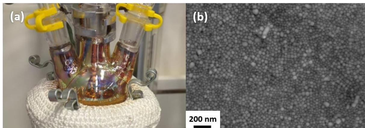
**Figure S1:** (a) Photograph of the occasionally occurring silver mirror and (b) SEM image of the resulting Ag nanoparticles.
