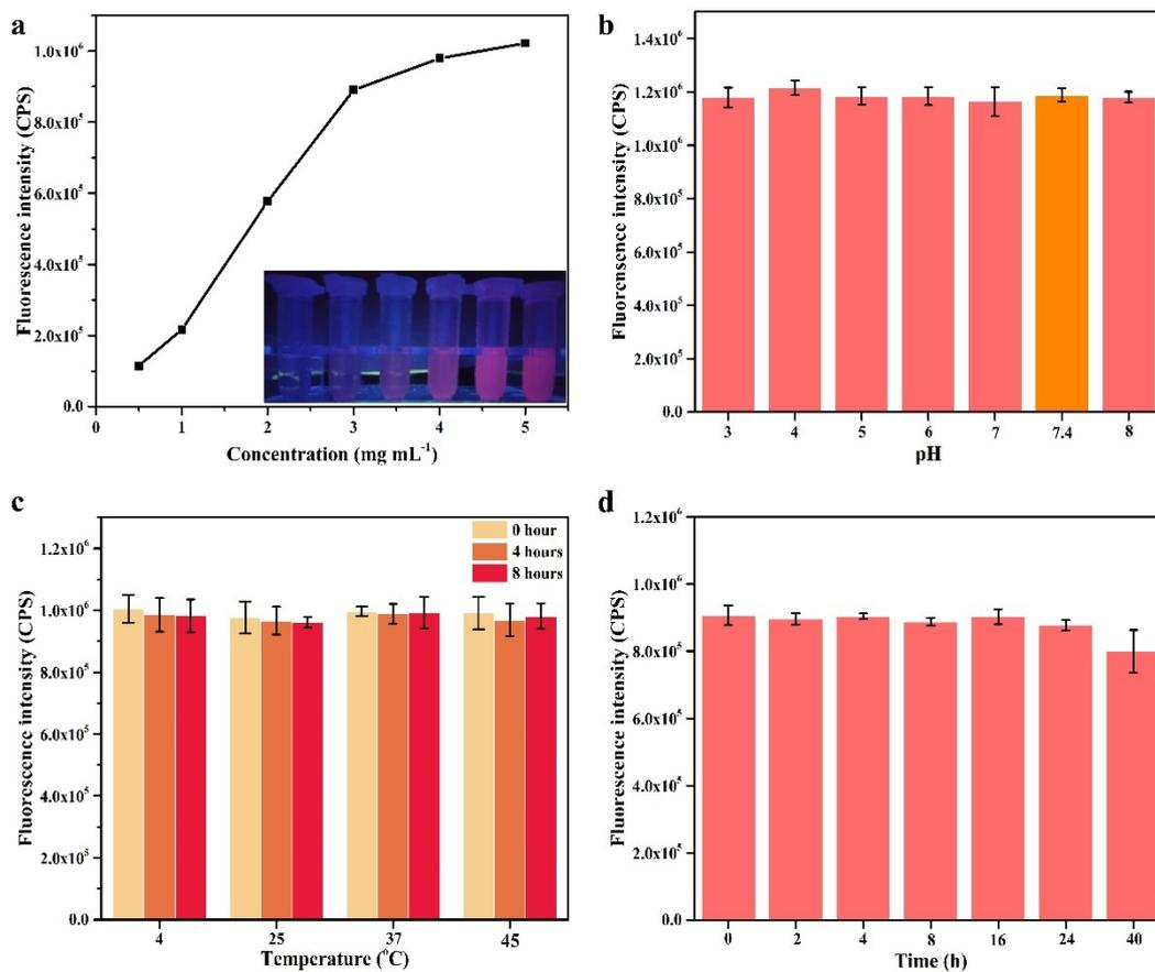
**Supplementary Figure 4. Optimization and Stability of Fluorescent Systems.** **a**, concentration investigation of ZIF-8@Ins-GOx/AuNCs. **b**, The pH stability of ZIF-8@Ins-GOx/AuNCs in the range of 3.0~8.0. **c**, The temperature stability of ZIF-8@Ins-GOx/AuNCs (4~45 °C). **d**, The study of photobleaching resistance.
