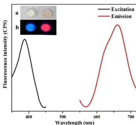
**Supplementary Figure 3. Excitation and emission spectra of ZIF-8@Ins-GOx/AuNCs.** Excitation and emission spectra of ZIF-8@Ins-GOx/AuNCs are shown. Inset images display ZIF-8 (left) and ZIF-8@Ins-GOx/AuNCs (right) under visible light (a) and UV lamp (b).
