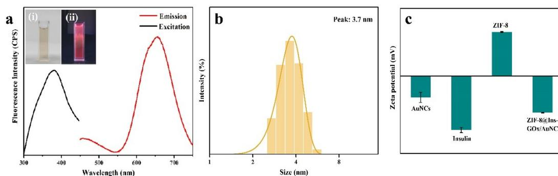
**Supplementary Figure 2. Characterization of AuNCs.** **a**, The fluorescence excitation and emission spectra of AuNCs. Inset images display the AuNCs solution under visible light (i) and under a UV lamp (365 nm) (ii). **b**, The size distribution of AuNCs. **c**, Zeta potential values for AuNCs, Insulin, ZIF-8, and ZIF-8@Ins-GOx/AuNCs nanocomposites.
