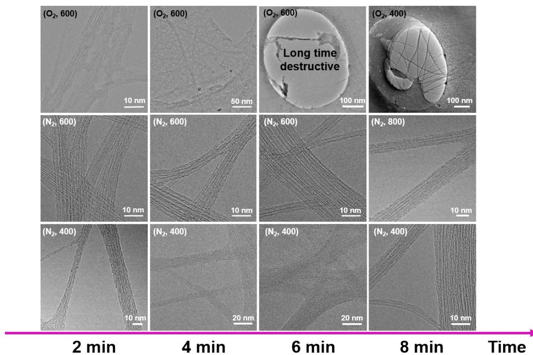
**Figure S2.** TEM images of CNTs under different RTP time ( $t= 2, 4, 6, 8$  min), temperature (400, 600, 800°C) and gas atmosphere (N<sub>2</sub> and O<sub>2</sub>).
