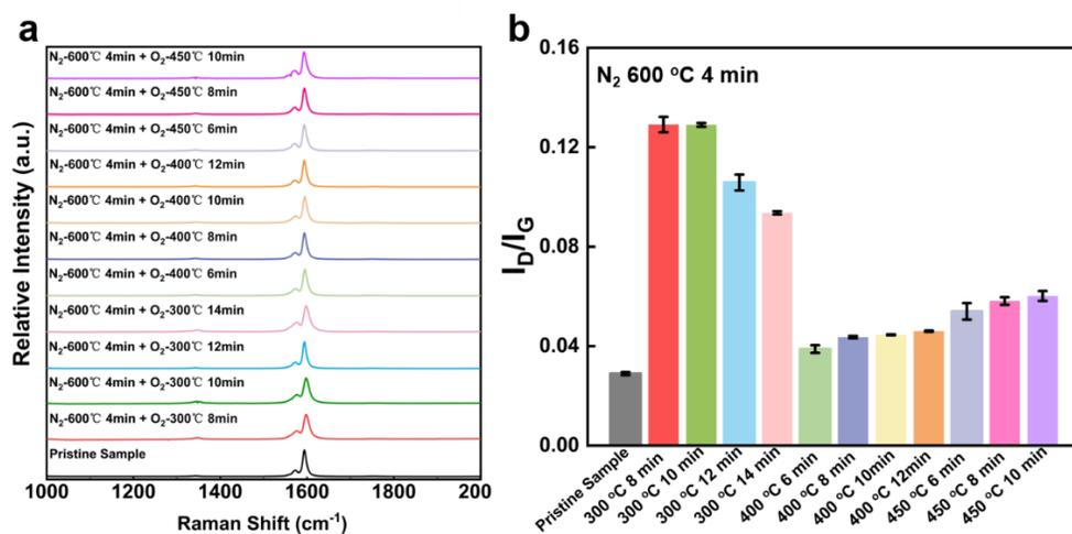
**Figure S3.** Detailed Raman results. (a) Raman full spectra under different RTP treatment conditions. (b) I<sub>D</sub>/I<sub>G</sub> defect ratio statistics under different treatment conditions.
