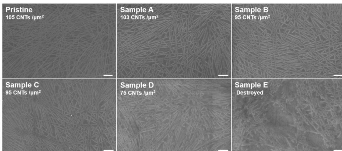
**Figure S4.** SEM characterization of the carbon nanotube network. (scale bar: 200 nm)
