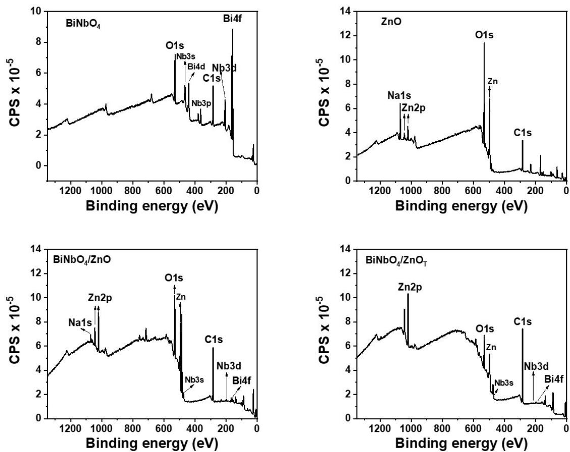
Figure S4. XPS survey spectra of ZnO, BiNbO<sub>4</sub>, BiNbO<sub>4</sub>/ZnO and BiNbO<sub>4</sub>/ZnO<sub>T</sub> samples.
