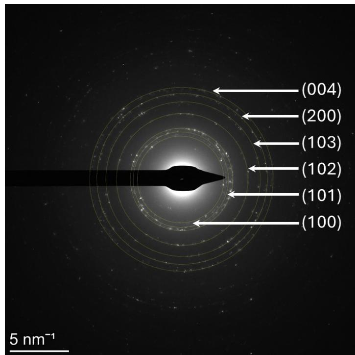
Figure S2. Pattern diffraction obtained from the selected area electron diffraction (SAED) of ZnO.
