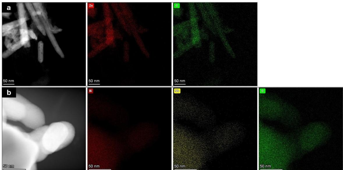
Figure S3. STEM images and elemental mapping of samples a) ZnO and b) BiNbO<sub>4</sub>.
