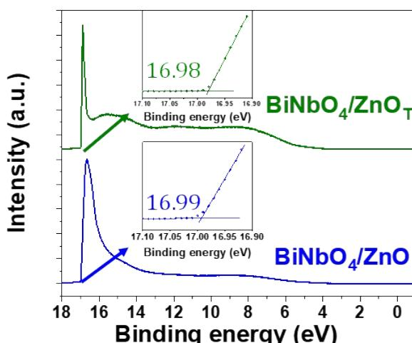
Figure S5. Ultraviolet photoelectron spectra (He-I) of BiNbO<sub>4</sub>/ZnO and BiNbO<sub>4</sub>/ZnO<sub>T</sub> samples.
