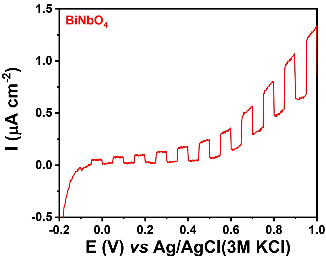
Figure S7. Chopped-light linear sweep voltammogram acquired using  $\text{BiNbO}_4$  film as the working electrode.  $\text{Ag}/\text{AgCl}$  (KCl 3M) was used as a reference, and a Pt wire as a counter electrode. An aqueous solution of 0.01 M  $\text{Na}_2\text{SO}_4$  was used as electrolyte. The scan rate was 50  $\text{mV s}^{-1}$ .
