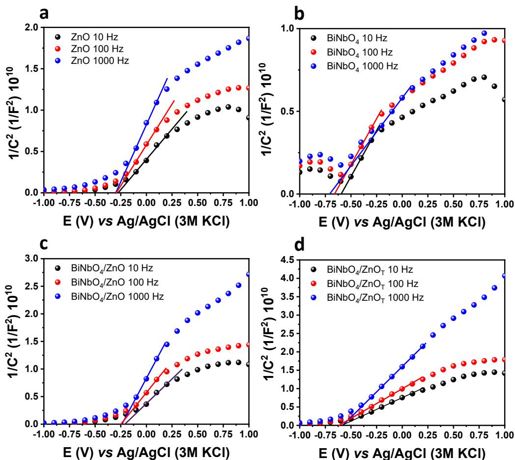
Figure S6. Mott-Schottky plots of ZnO (a), BiNbO<sub>4</sub> (b), BiNbO<sub>4</sub>/ZnO (c) and BiNbO<sub>4</sub>/ZnO<sub>T</sub> (d)
