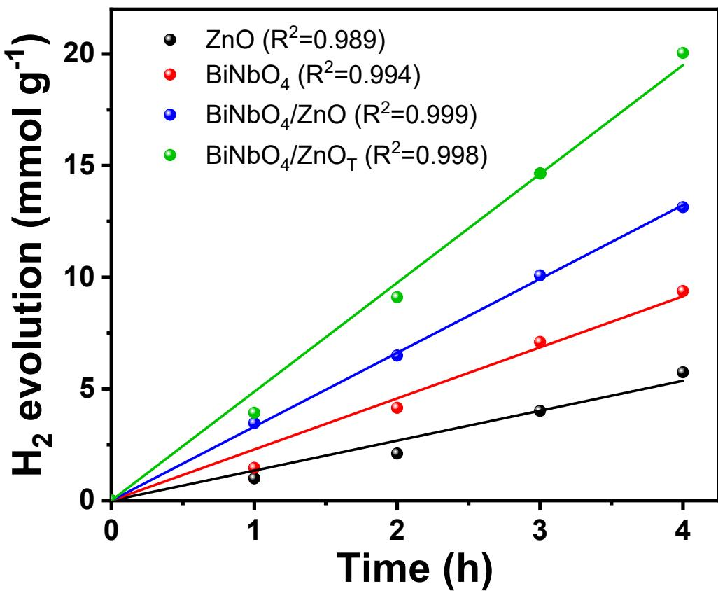
Figure S8.  $H_2$  evolution of ZnO,  $BiNbO_4$ ,  $BiNbO_4/ZnO$  and  $BiNbO_4/ZnO_T$  films under UV light.
