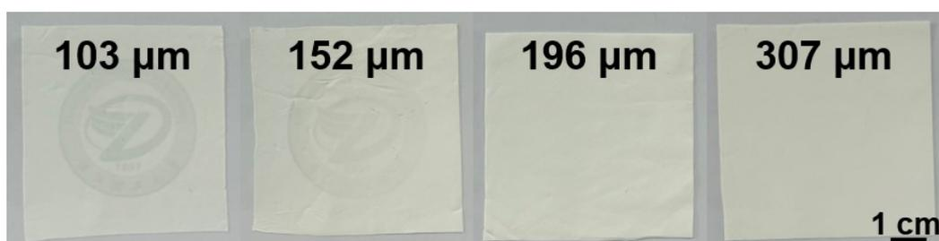
**Fig. S8.** Optical pictures of PHB-4% fabrics with different thickness.
