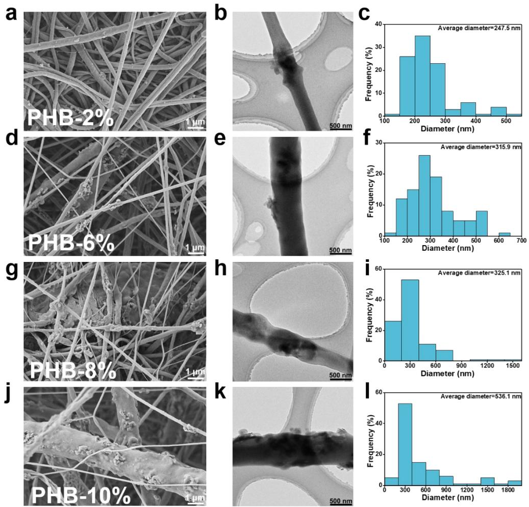
**Fig. S1.** SEM, TEM, and diameter distribution images of PHB-2% (a, b, c), PHB-6% (d, e, f), PHB-8% (g, h, i), and PHB-10% (j, k, l) fabrics.
