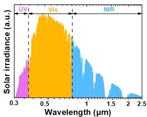
**Fig. S6.** Spectra of solar irradiance (plotted by AM 1.5G, global tilt).
