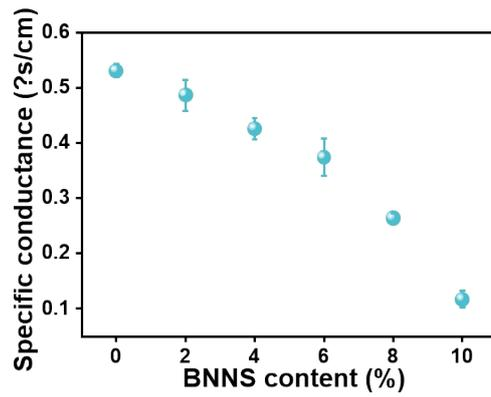
**Fig. S3.** The specific conductance of PVDF-HFP solution with different BNNs content.
