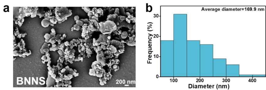
**Fig. S2.** SEM image (a) and diameter distribution (b) of BNNS.
