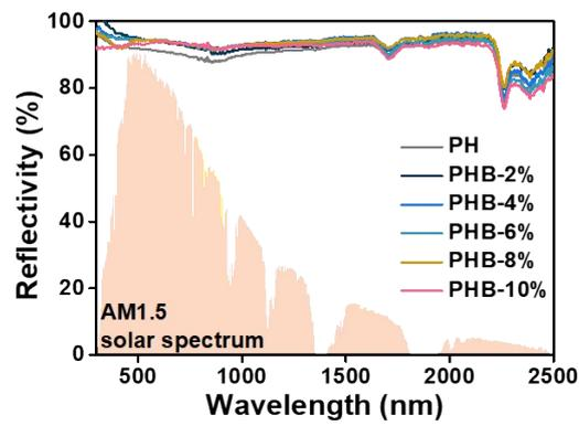
**Fig. S4.** The solar reflectivity spectra of the fabrics with different BNNs content.
