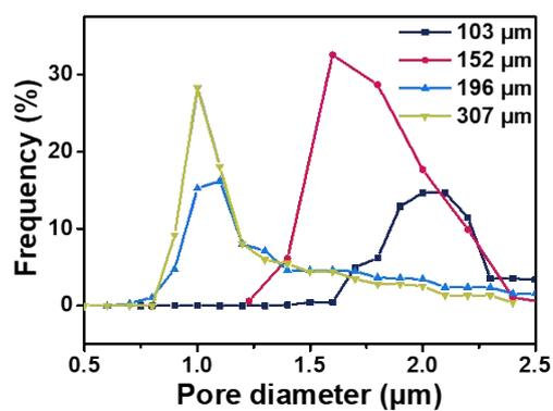
**Fig. S7.** Pore diameter distribution of the PHB-4% fabrics with different thickness.
