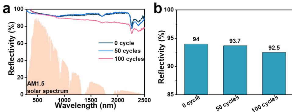
**Fig. S11.** The solar reflectivity spectra (a) and calculated value (b) of the PHB-4% fabric undergo difference washing cycles.
