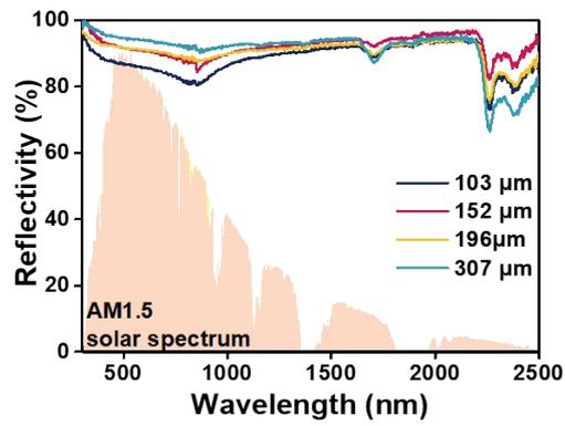
**Fig. S9.** The solar reflectivity spectra of the PHB-4% fabrics with different thickness.
