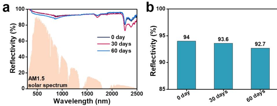
**Fig. S10.** The solar reflectivity spectra (a) and calculated value (b) of the PHB-4% fabric under direct sunlight for different days.
