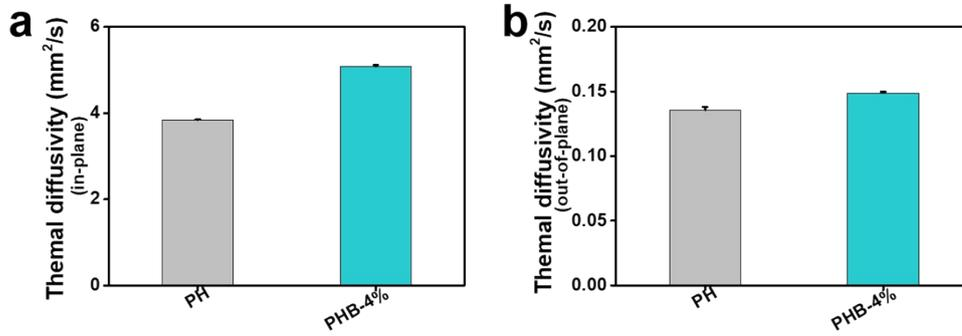
Fig. S13. (a) In-plane and (b) out-of-plane thermal diffusivity of PH and PHB-4% fabrics.
