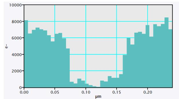
Fig. S 6 Profile plot across the oxidized (beam-affected) area. Multiple profile plots were acquired, and the diameter of the affected region was extracted from these measurements.
