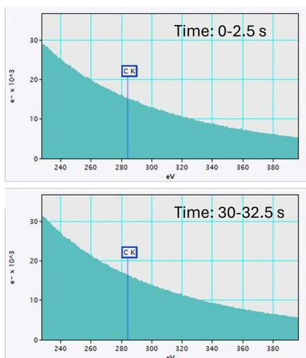
Fig. S 1 Signal from the carbon energy loss range at the beginning of a time series and after 30 seconds of electron beam exposure, corresponding to an accumulated dose of approximately  $\sim 5 \cdot 10^8 e^-/\text{\AA}^2$
