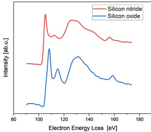
Fig. S 4 Standards for the silicon nitride and silicon oxide signal<sup>19</sup>.
