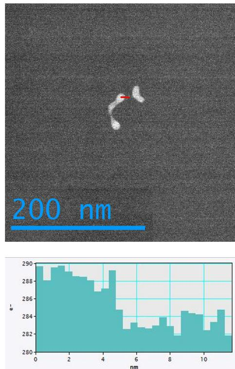
Fig. S 3 STEM image of the membrane with surface contamination. The corresponding intensity profile was acquired along the red line shown in the image. The pixel size is 0.86 nm.
