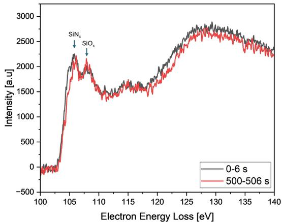
Fig. S 5 Signal from the membrane (adjacent to a channel), where no water is present. The measurement was acquired at a dose rate of  $8 \cdot 10^6 \text{ e}^- / (\text{\AA}^2 \cdot \text{s})$ .
