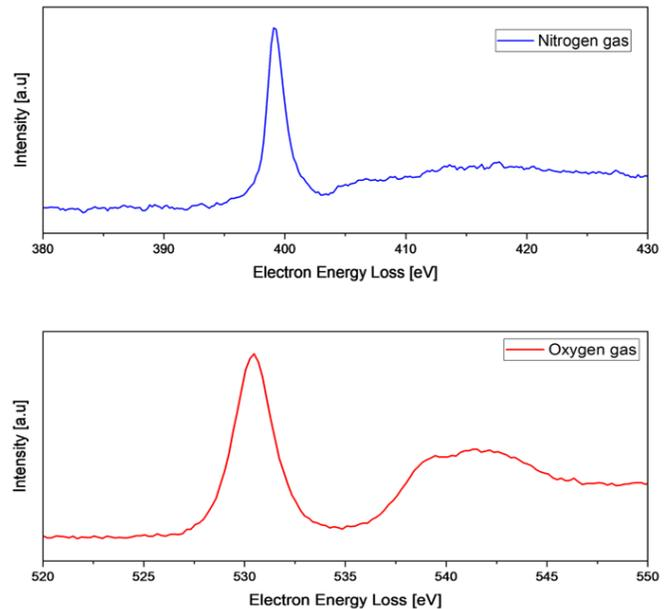
Fig. S 7 Standards for the nitrogen gas<sup>19</sup> and oxygen gas from the Gatan EELS Atlas.
