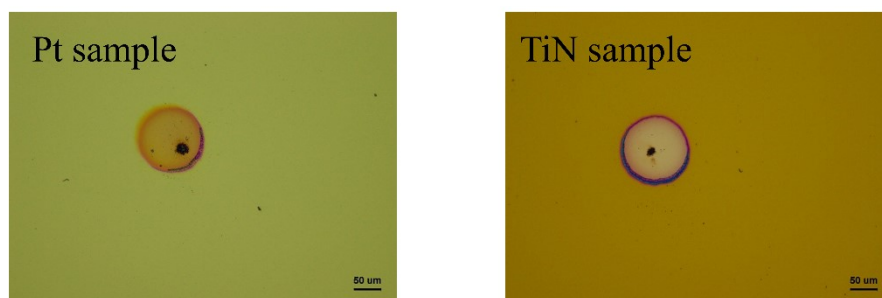
S. 3. Electrode images after failure, (left) Pt sample and (right) TiN sample.
