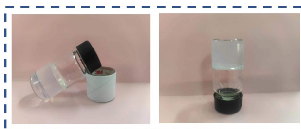
Figure S2. Photographs of PVA/Borax organohydrogels in tilted and inverted small bottles.
