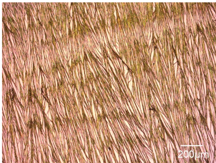
Figure S3. Optical microscope image of the ordered microwire arrays (OMAs) obtained by self-ssembling of AYM on fully cured PDMS substrate.
