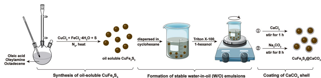
Fig. S1 Synthesis diagram of \text{CuFe}_2\text{S}_3@\text{CaCO}_3 nanocomposites.
