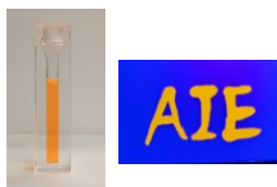
Figure S.49 Appearance of DPRP-SNAFL. Left: In solution (20 \mu M in acetone) under ambient light. Right: Adsorbed on silica TLC plate illuminated by 365 nm light source.
