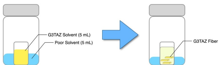
Figure S1. Schematic diagram of vapour diffusion method for the synthesis of crystalline G3TAZ powder.
