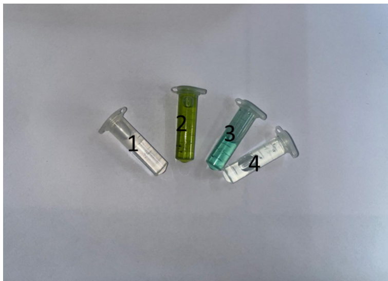
Fig. S10 Change in color with different concentrations of resorcinol 0.1mM (1) TMB+H 2 O 2 + Resorcinol (2,3and 4) TMB+ H 2 O 2 + NPs+no resorcinol, 0.2mM Resorcinol, 0.8mM Resorcinol respectively.
