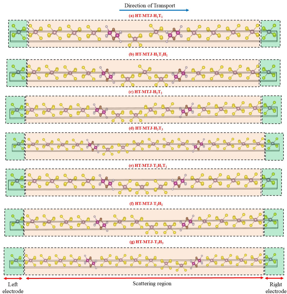
Figure S22: Schematic illustration of device configurations incorporating HT-MTJs, which denote heterophase (1T/2H) MoS 2 tunnel barriers. For HT-MTJ devices, the notation (H/T) represents the stacking sequence of 2H and 1T layers from left to right across the tunnel barrier, with numbers indicating multiple layers of each phase.
