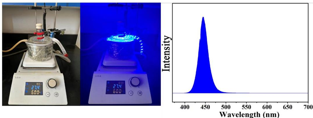
**Figure S1.** Devices for the reactions and the emission spectrum of blue LEDs.
