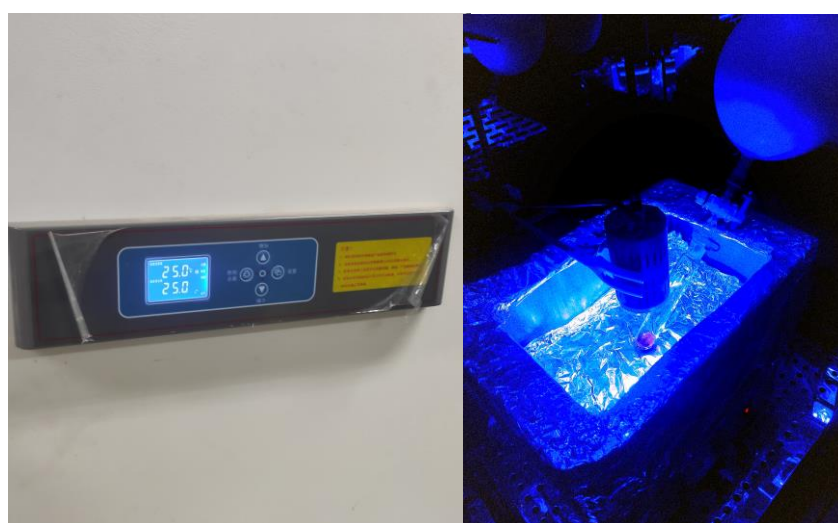
Figure S1. Reaction equipment and light source ( \lambda_{\text{peak}} = 454 \text{ nm} ).
