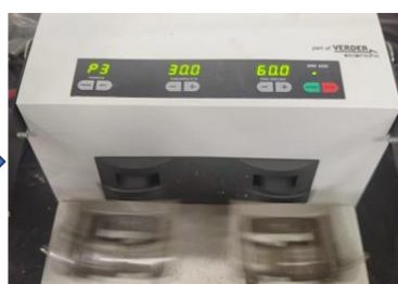
Step 2: Ball milling for 60 min (30 Hz)
