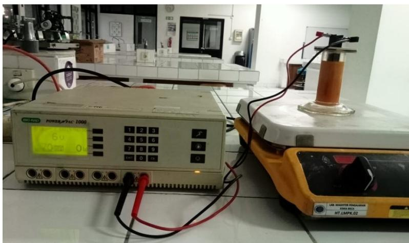
**Figure 3.** Scale-up reaction set up for electrochemical amidation.
