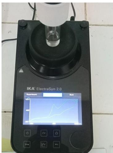
**Figure 7.** Cyclic voltammetry experiments.
