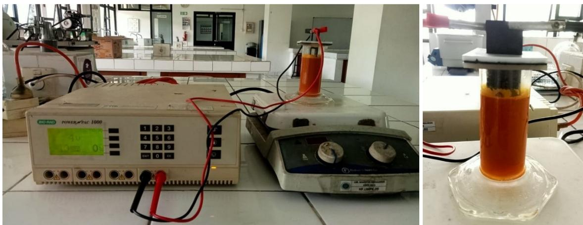
**Figure 6.** Scale-up reaction set up for electrochemical condensation.
