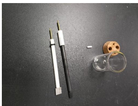
Figure S1. The materials used to make the electrolytic cell for the synthesis of quinazolin-4(3 H )-one
