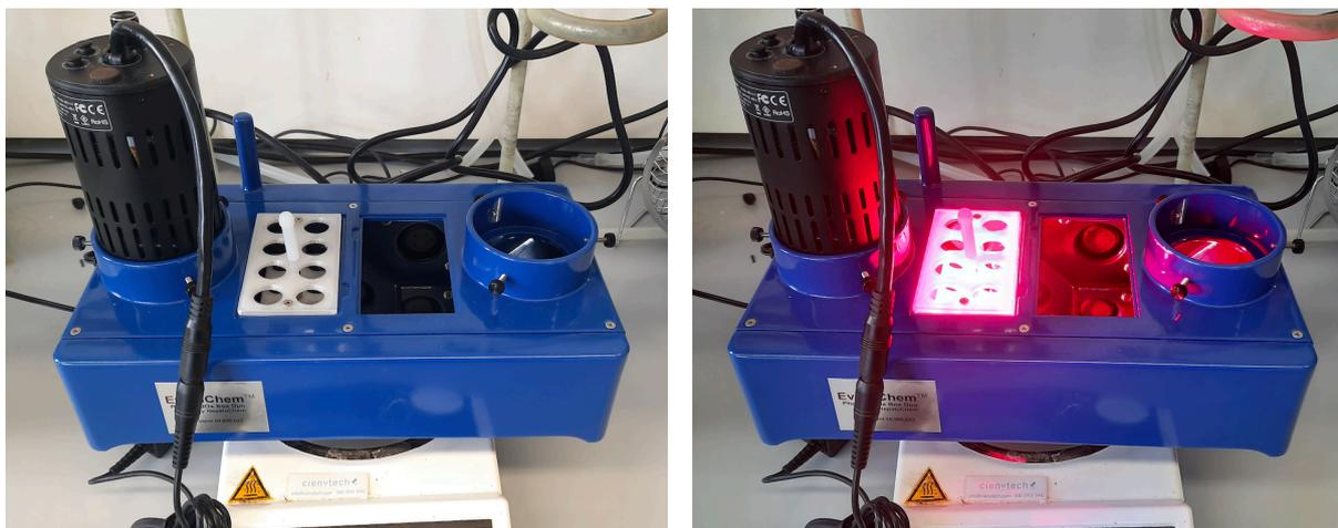
**Figure S3.** Pictures of the photochemical set up with one operative chamber (light off or on).
