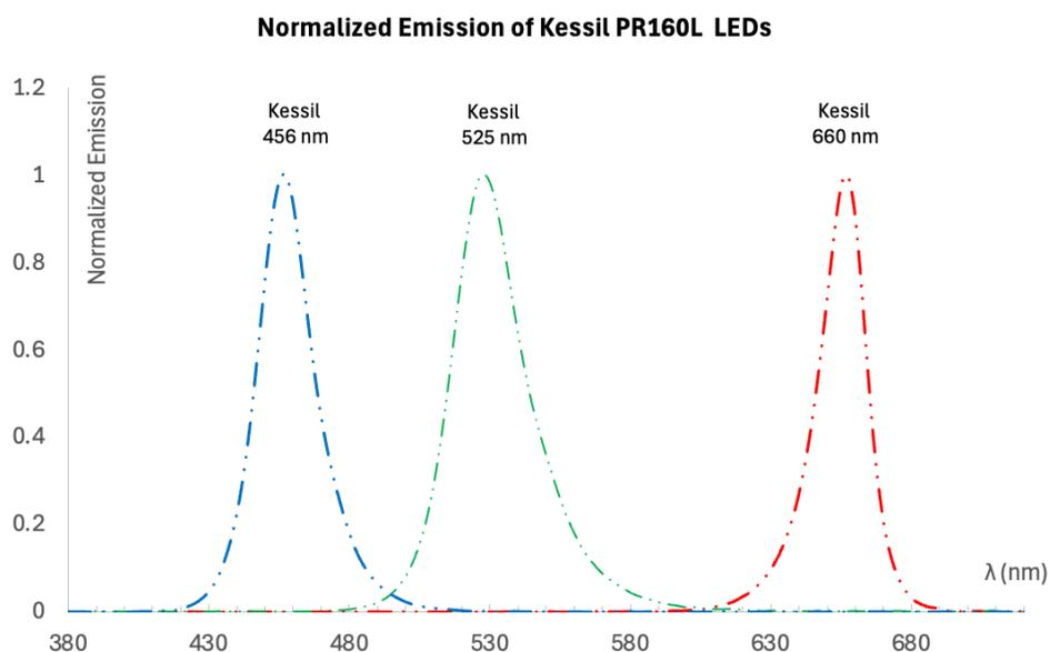
**Figure S1.** Recorded normalized emission of the Kessil LED light sources employed in this study.
