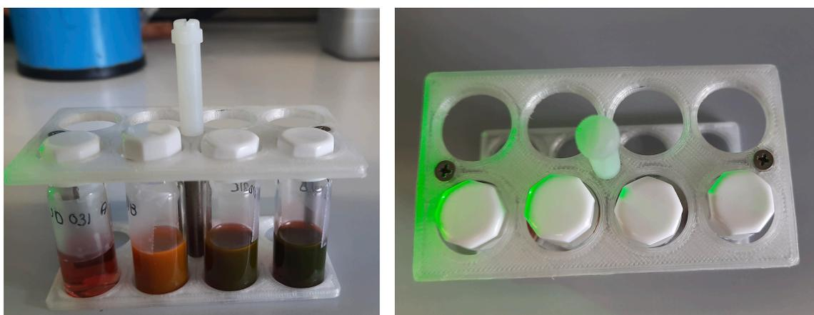
**Figure S4.** Pictures of the reaction vials and sample holder that is located in the chamber; front (left) or top view (right).
