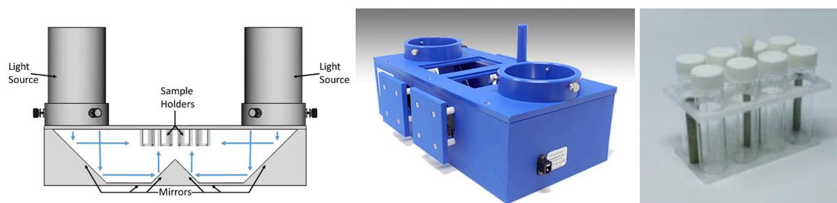
**Figure S2.** Schematic representation (left), picture of the photoreactor (center) and sample holder for 8 mL vials (right) provided by HepatoChem.
