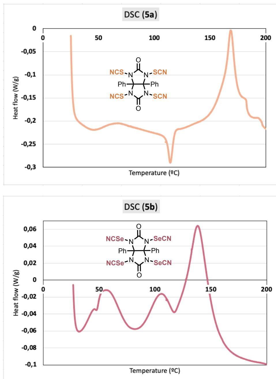
**Figure S1.** DSC analysis of reagents **5a** and **5b**
