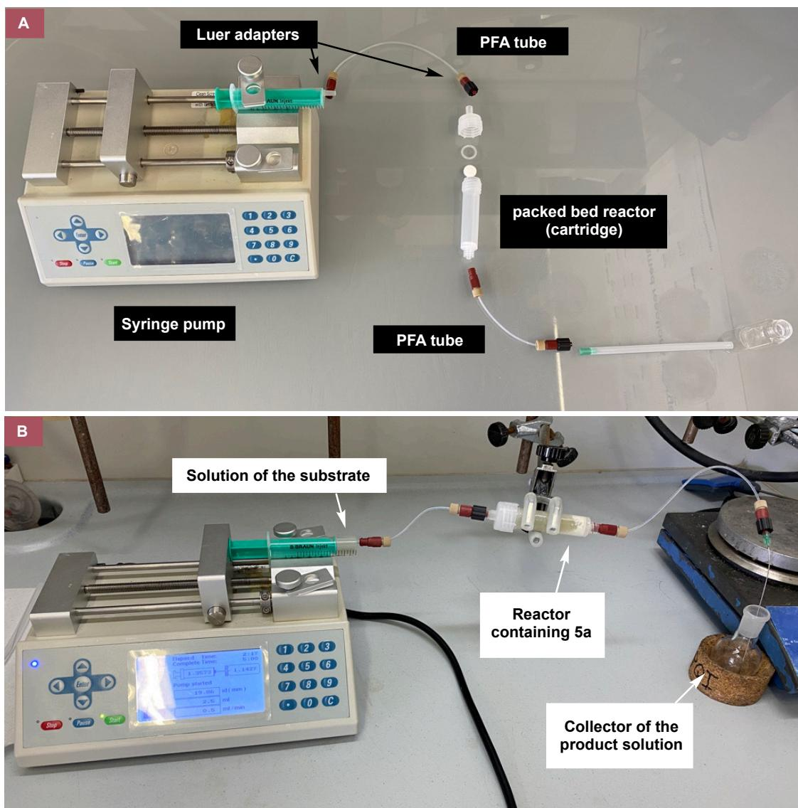
**Figure S7.** (A) Set-up description. (B) Schematic representation of the reaction procedure using a flow chemistry setup
