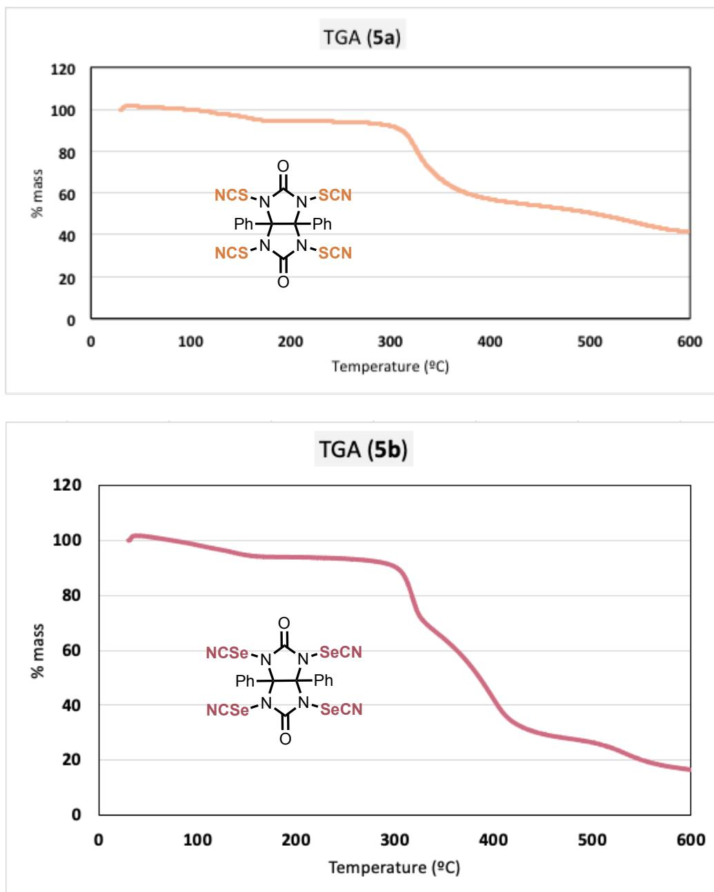
**Figure S2.** TGA analysis of reagents **5a** and **5b**. 5% weight decomposition (**5a**) = 167 °C; 5% weight decomposition (**5b**) = 143 °C
