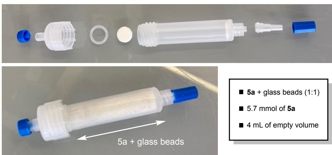
**Figure S6.** Packed bed reactor used in this study
