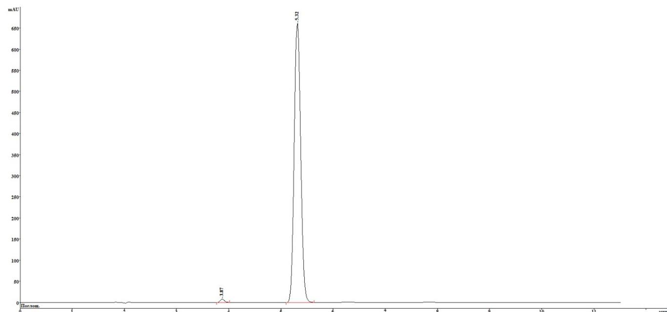
**6o.** HPLC conditions: Chiralpak AD-H, *i*-PrOH/*n*-hexane 5 : 95, flow rate = 1.5 ml/min.
