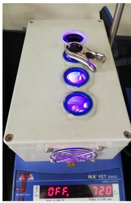
Figure S1. Photoreactor used in this research (40 W purple LEDs)
