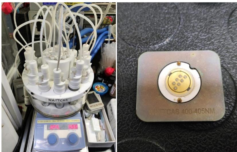
**Figure S1.** Photo reactor device and 405 nm 10 W blue LED chip
