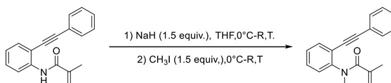
**Scheme S3.** Synthesis of N-methyl-N-(2-(phenylethynyl)phenyl)methacrylamide
