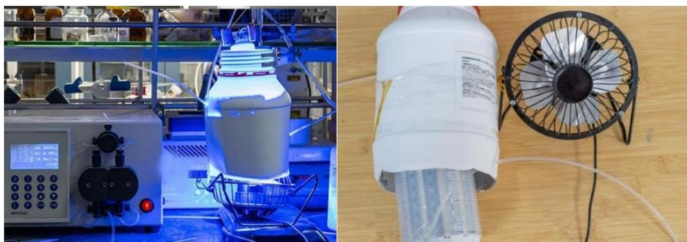
**Figure S2.** Example figure of gram scale flow reactor of photoreactions
