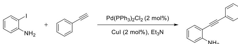
**Scheme S1.** Synthesis of 2-(phenylethynyl)aniline
