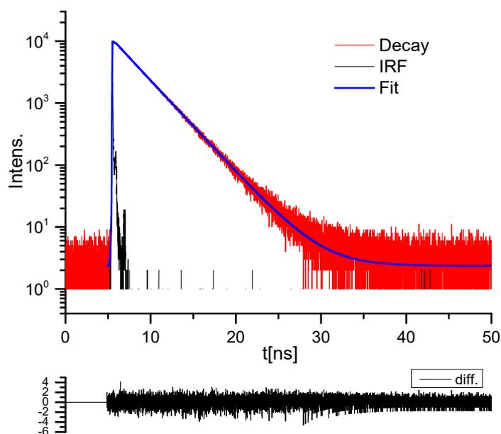
**Fig. S44.** Kinetics of fluorescence decay of compound **8b** (L) in acetonitrile ( $\tau = 2.93$  ns).
