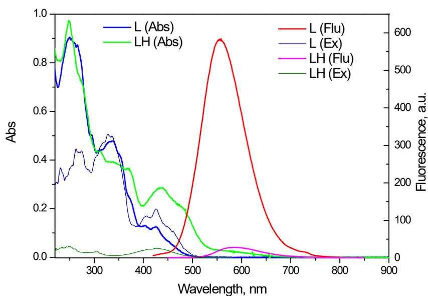
**Fig. S41.** Absorption (Abs), fluorescence (Flu) and fluorescence excitation (Ex) spectra of compound **8a** (L) in acetonitrile and (LH) in acidified acetonitrile ( $\sim 0.02$  M  $\text{HClO}_4$ ).
