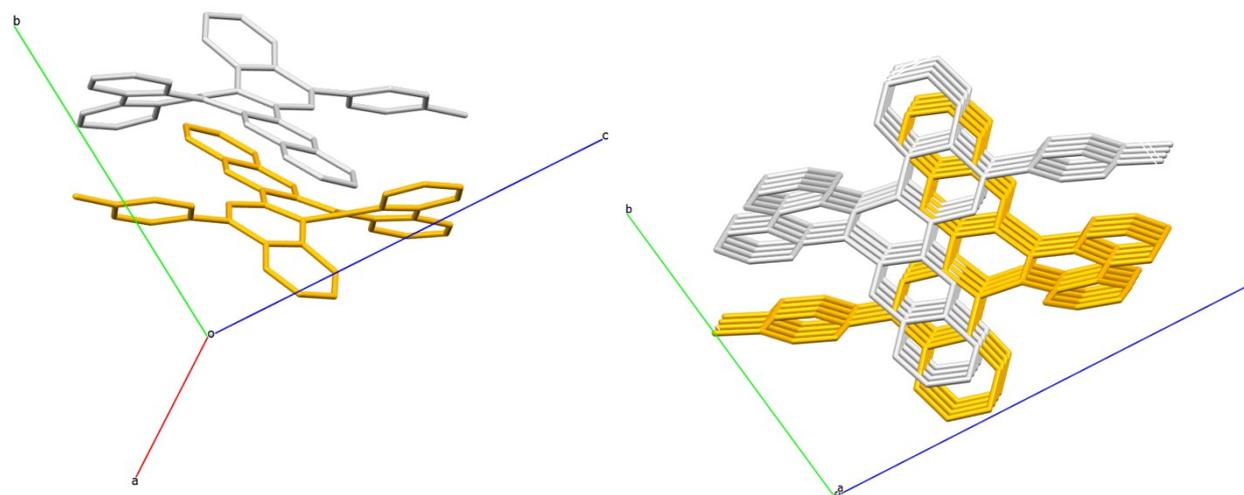
**Fig. S36.** Crystal unit cell and packing of **8a** (molecules are colored by symmetry operation).
