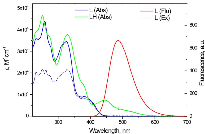
**Fig. S43.** Absorption (Abs), fluorescence (Flu) and fluorescence excitation (Ex) spectra of compound **8b** (L) in acetonitrile and (LH) in acidified acetonitrile ( $\sim 0.02$  M  $\text{HClO}_4$ ).
