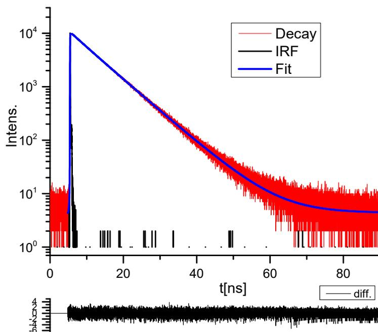
**Fig. S48.** Kinetics of fluorescence decay of compound **8c** (L) in *n*-heptane ( $\tau = 7.25$  ns).
