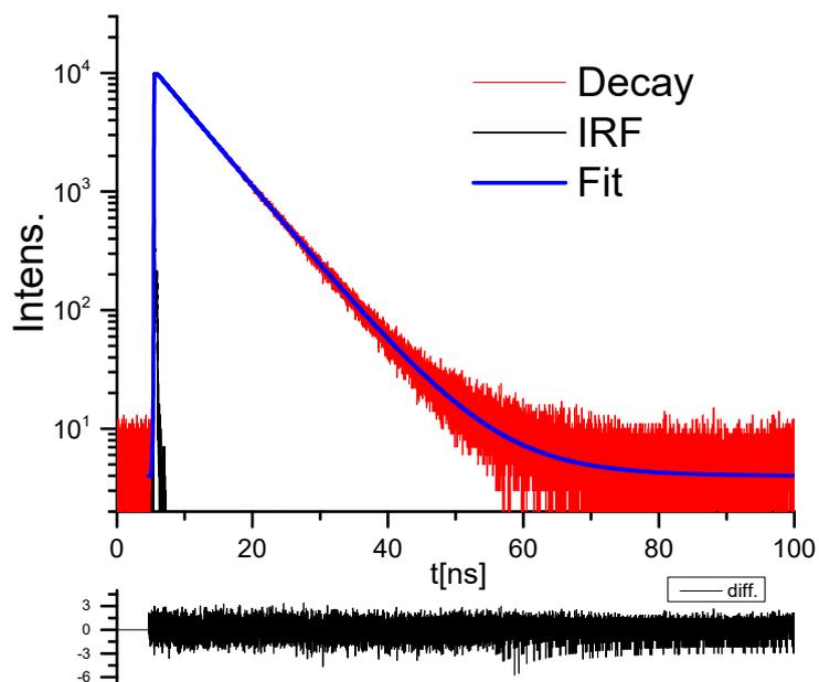
**Fig. S50.** Kinetics of fluorescence decay of compound **8c** (L) in chloroform ( $\tau = 6.48$  ns).
