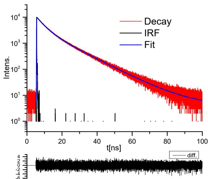
**Fig. S42.** Kinetics of fluorescence decay of compound **8a** (L) in acetonitrile ( $\tau_1 = 12.92$  ns,  $\tau_2 = 4.075$  ns).
