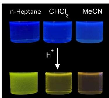
**Fig S52.** Solutions of helicene **8c** without acid (top) and with CF<sub>3</sub>COOH (bottom) under UV irradiation (365 nm).
