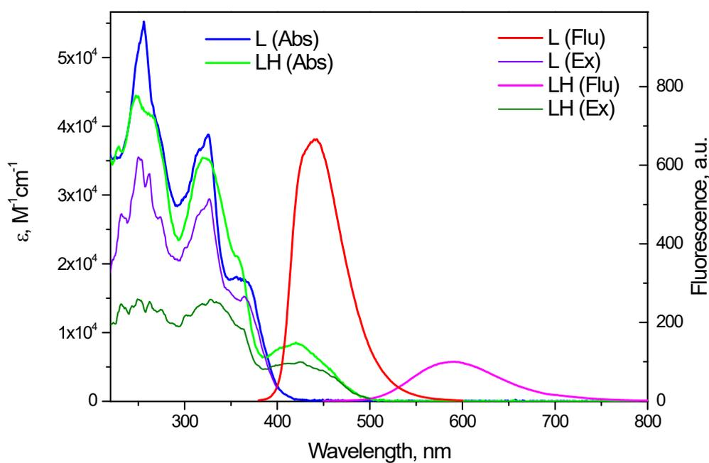
**Fig. S45.** Absorption (Abs), fluorescence (Flu) and fluorescence excitation (Ex) spectra of compound **8c** (L) in acetonitrile and (LH) in acidified acetonitrile ( $\sim 0.02$  M  $\text{HClO}_4$ ).
