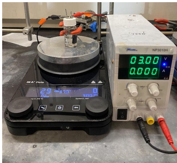
Figure S1. Photograph of the in-house electrolytic cell used for the reactions (0.5 mmol scale).
