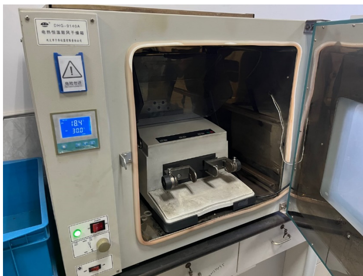
Figure S1 Mix-miller placed in a thermostat oven to ensure the starting temperature.
