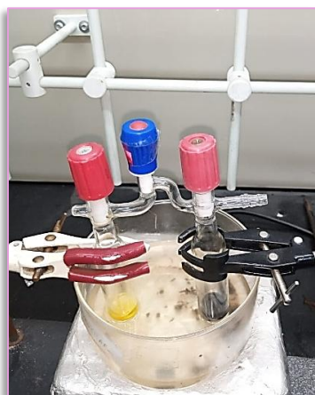
Figure S1: Experimental bridge-shaped Schlenk tube setup for hydrogenation of styrene using Pd/C and generated H_2 from annulation of 2-aminobenzyl alcohol with 1-phenylethanol to form quinoline derivatives.
