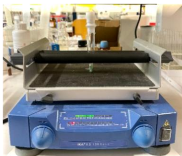
Figure S13. Orbital shaker used to stir the reaction at room temperature
