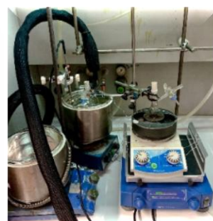
Figure S14. The setup for temperature optimization
