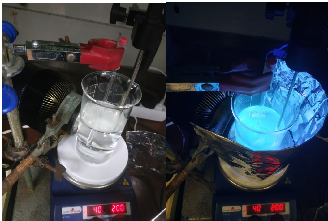
Figure S3. Photochemical set-up with heating.
